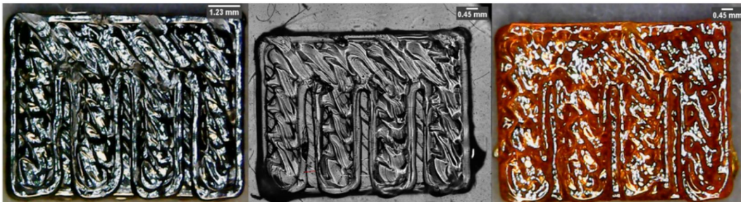
Figure 11 Shows the fidelity of pattern transferring using super soft lithography. From left to right, ABS master mold, hard-PDMS mold and candy mold.
