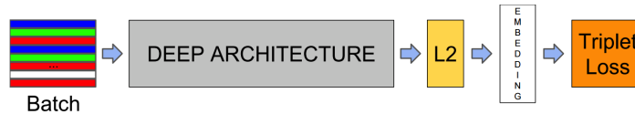
Figure 2.10: Outline of the FaceNet deep neural network architecture as described in [9]. This network consists of a batch input, a deep CNN followed by l_2 normalization, and finally a triplet loss during training.
