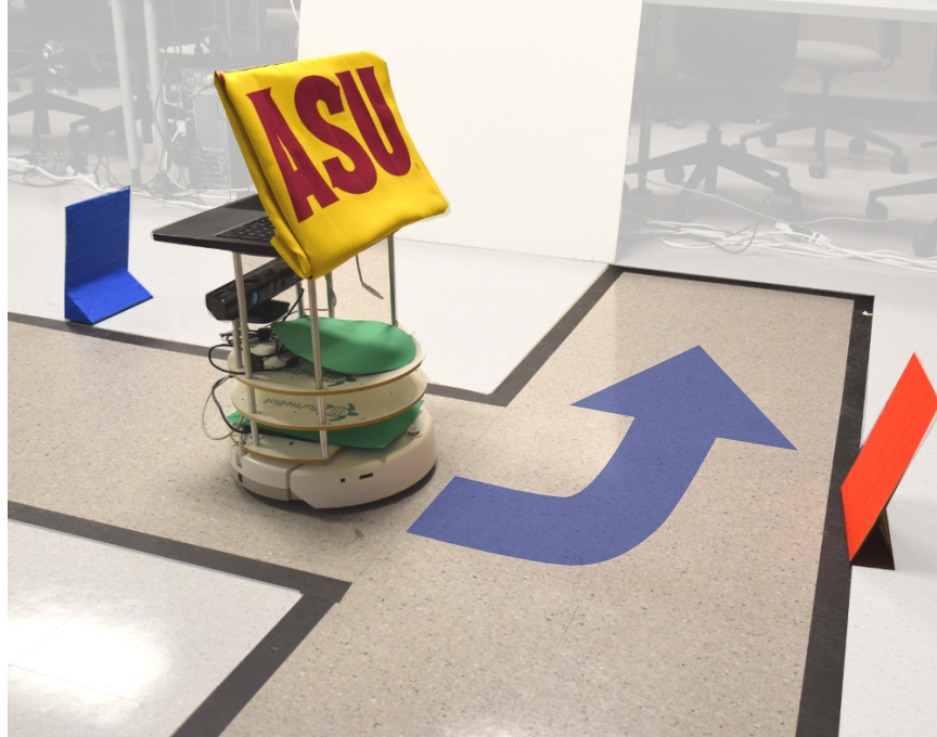
Figure 1.1: A Robot Moving to a 3-way Junction. Before Reaching the Intersection, the Robot Is Provided Information about Which Direction to Turn. This Is Realized via a Colored Sign (Blue or Green Rectangle). At the Intersection, the Robot Should Make a Decision to Turn Based on the Previously Observed Signal.
