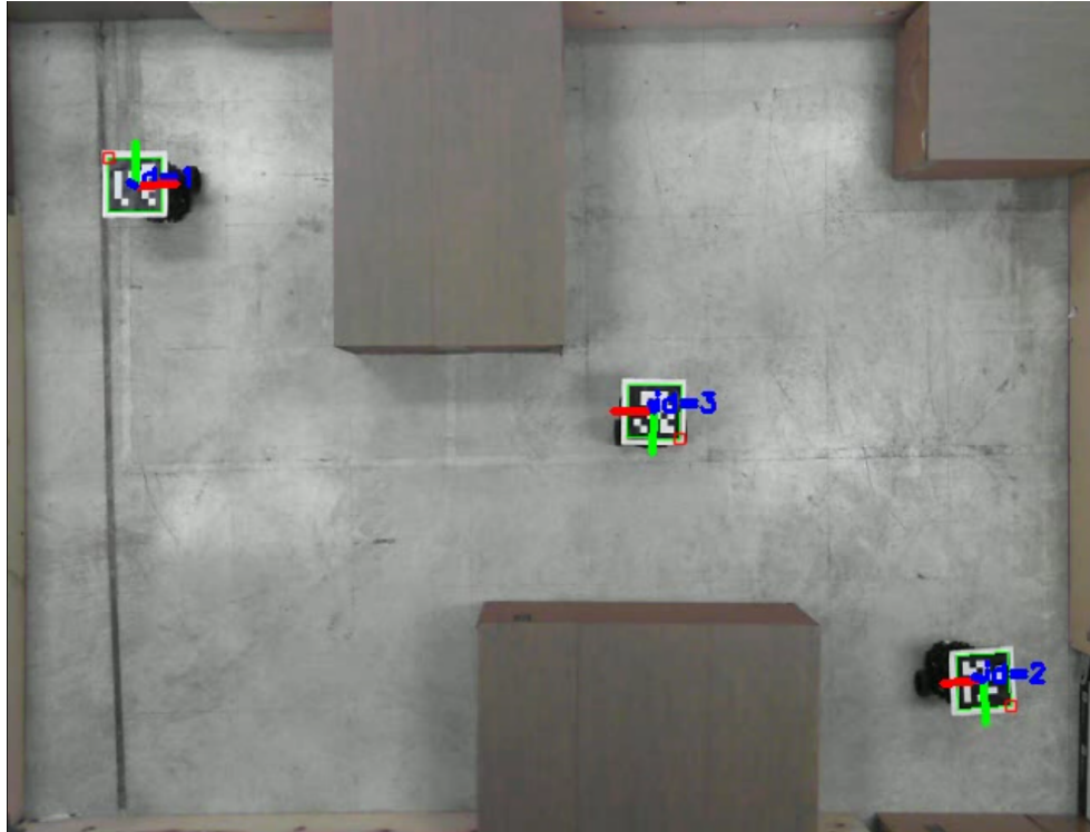
Figure 7.12: The experimental arena with obstacles. To minimize early robot interaction, the robots were placed in specific starting locations. For consistency in testing, the same positions were used for each trial.
