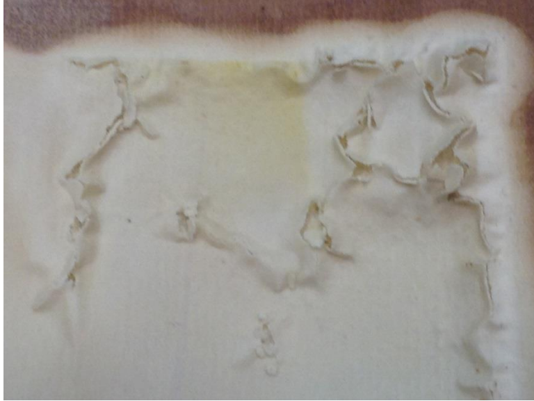
Figure B.2. Membrane cracking observed during operation with a 6-hr HRT and using a 200-mM NaCl catholyte and 20 \text{ cm}^3 \text{ min}^{-1} air flow rate.
