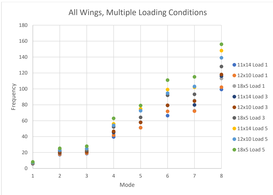
Figure 22: Modal Analysis for Three Wing Designs and Three Loading Cases
