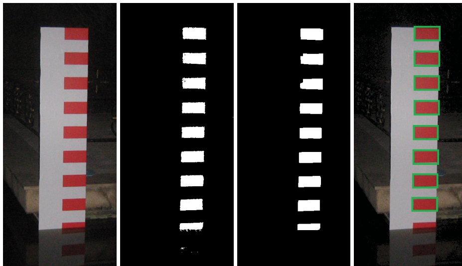
Figure 5.6: Detect watermarks from the panel, and then use Scale Adaptive Color FAST Affine Template matching to detect each water mark
