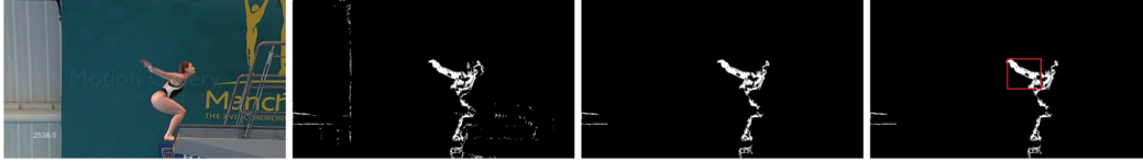
Figure 3.12: From left to right: 1. Original RGB image; OF obtained from RGB image; 2. extracting MSR candidates; 3. Discarding insignificant MSR candidates; 4. Keep the most motion salient region (the red rectangle is the selected MSR)
