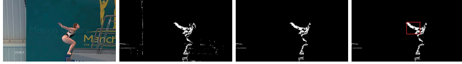
Figure 3.13: An outline of our method to select one MSR in the human body. From Left to Right: the result of step 1 - extracting MSR candidates, the result of step 2 - discarding the small MSR candidates, and the result of step 3 - selecting the most salient motion region (the red rectangle).
