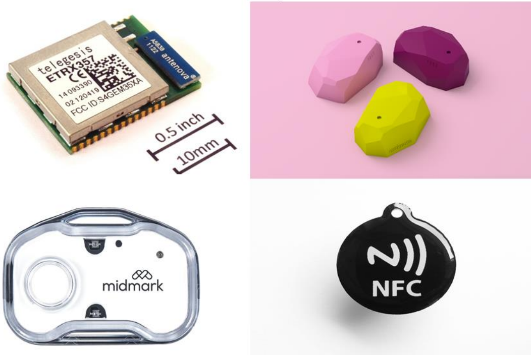
Figure 1: RTLS Tags. top-left: ZigBee (Wikipedia.org); top-right: Bluetooth (Estimote.com); bottom-left: RFID (Midmark.com); NFC (Wikimedia.org)
