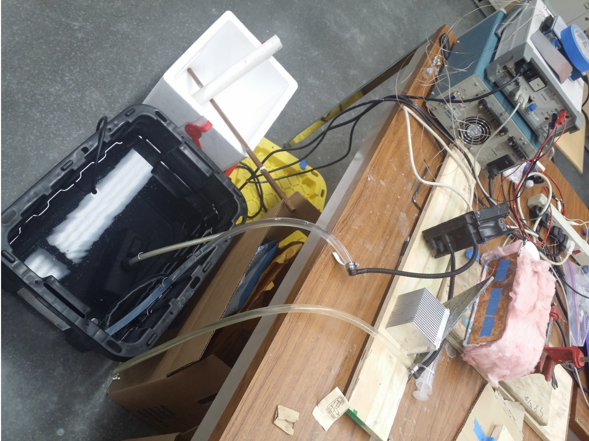
Figure 3.3: Image Showing the Physical Setup of the Experiment including the Water Cooling Pump and Water Reservoir.
