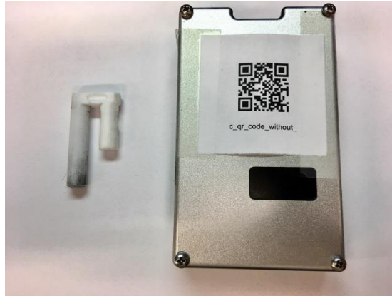
Figure 4-1. The schematic [136] (a) and the appearance of the VOC replaceable cartridge and device.
