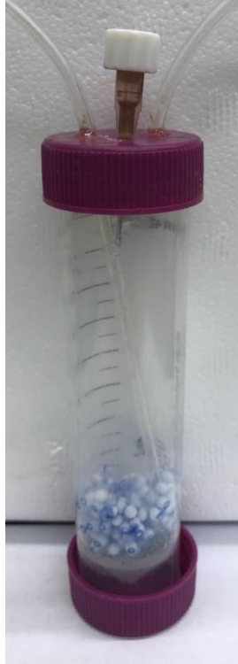
Figure 2-2. The actual look of the extraction column.
