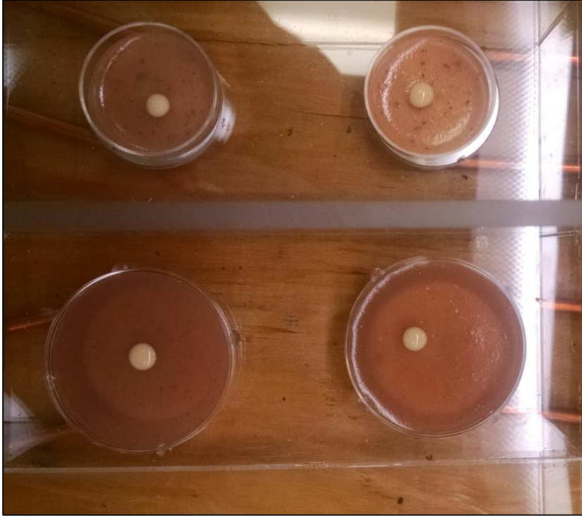
Figure 4.2. My thermal arena consisted of a Plexiglas container that consisted of 6 independent lanes by running copper tubing below small aluminum plates. Each lane within the arena had two aluminum plates on opposite ends of the lane where I could place an agar-filled petri dish with a drop of yeast. Flies could fly and lay their eggs in either the 16°C petri dish or the 25°C petri dish. Flies in the low-space treatment chose between 35mm diameter patches (top) while flies in the large space treatment chose between 50mm diameter patches (bottom). The total amount of yeast present in patches was constant between treatments.
