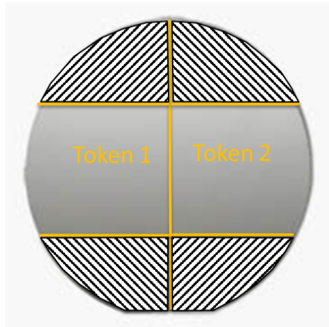
Fig. 3.1 Schematic of the two tokens obtained from each wafer after cleaving. The dimensions and shape of the tokens were chosen in order to facilitate the handling during the subsequent chemical treatments and limit the breakages.
