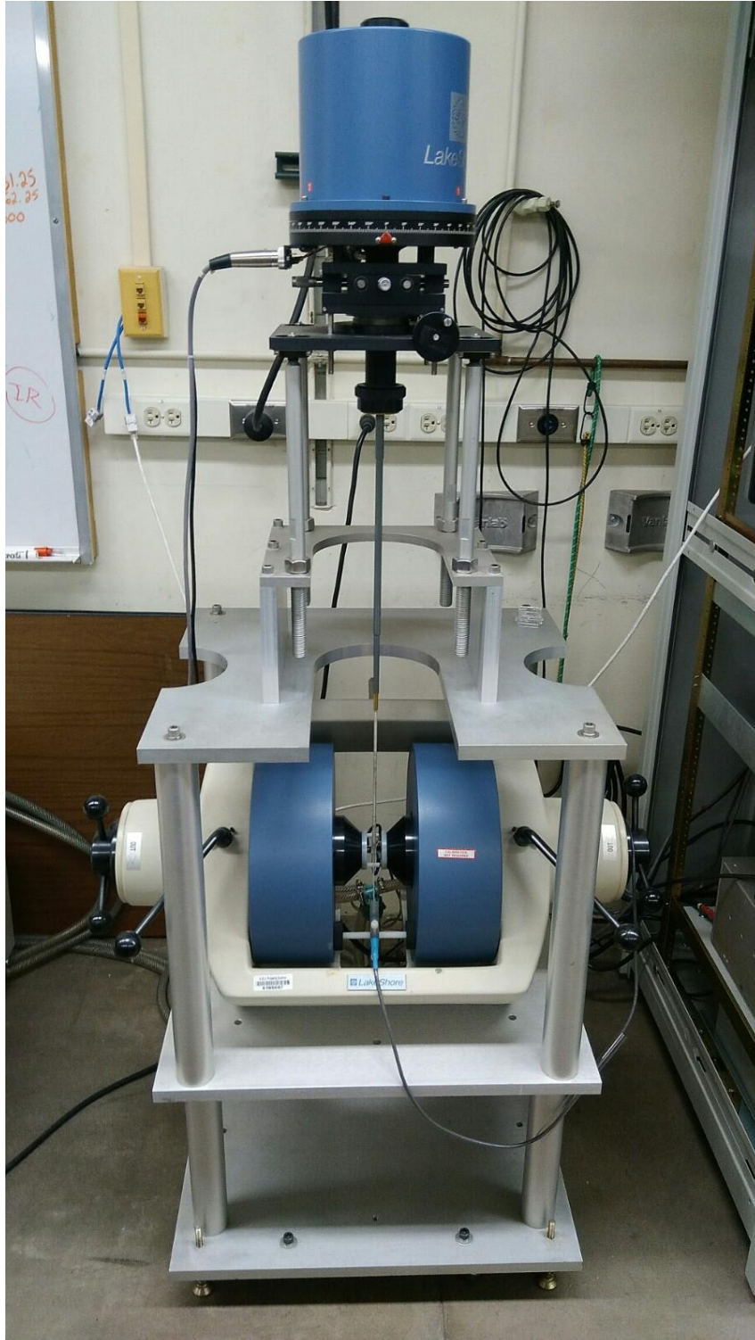
Figure 2.9: Photo of the Lakeshore 7304 VSM in our lab.
