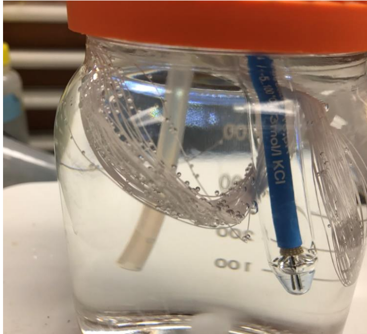
Figure 4.10. Bubble formation observed on the external surface of a closed-end HFM receiving pure CO 2 .
