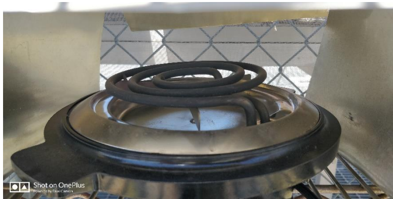
Figure 2.7 The burner coil used as an 880 W step.
