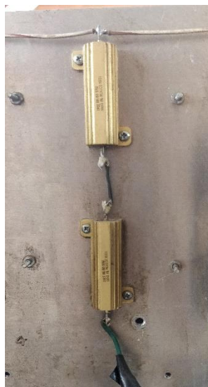
Figure 2.8 A set of resistors used as a 72 W step.
