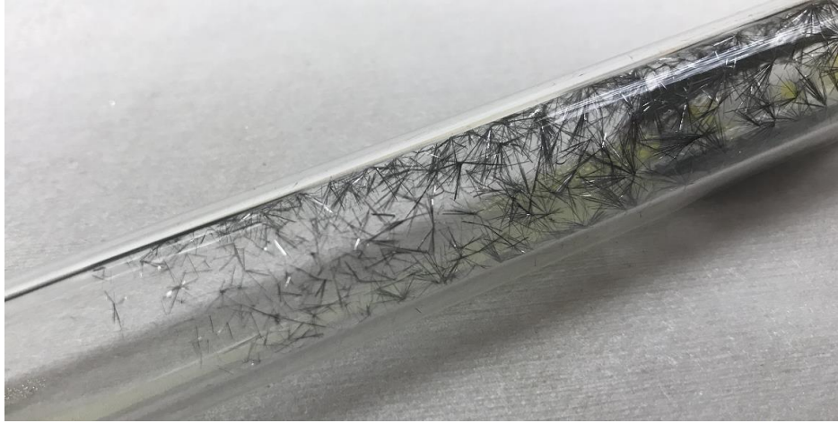
Figure 6.2 As grown \text{Nb}_{(1-x)}\text{Ti}_x\text{S}_3 ( x = 0.66 ) crystals on the interior wall of a quartz ampule.
