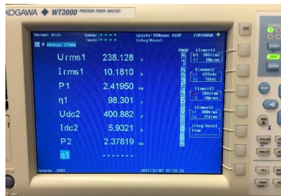
Figure 2.30 Circuit efficiency measurement at 2.4 kW
