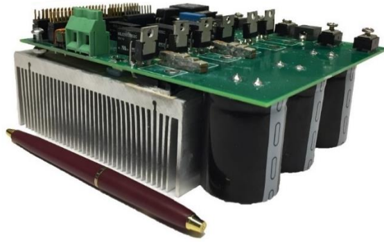
Figure 2.22 Photograph of the ZVT full-bridge converter prototype
