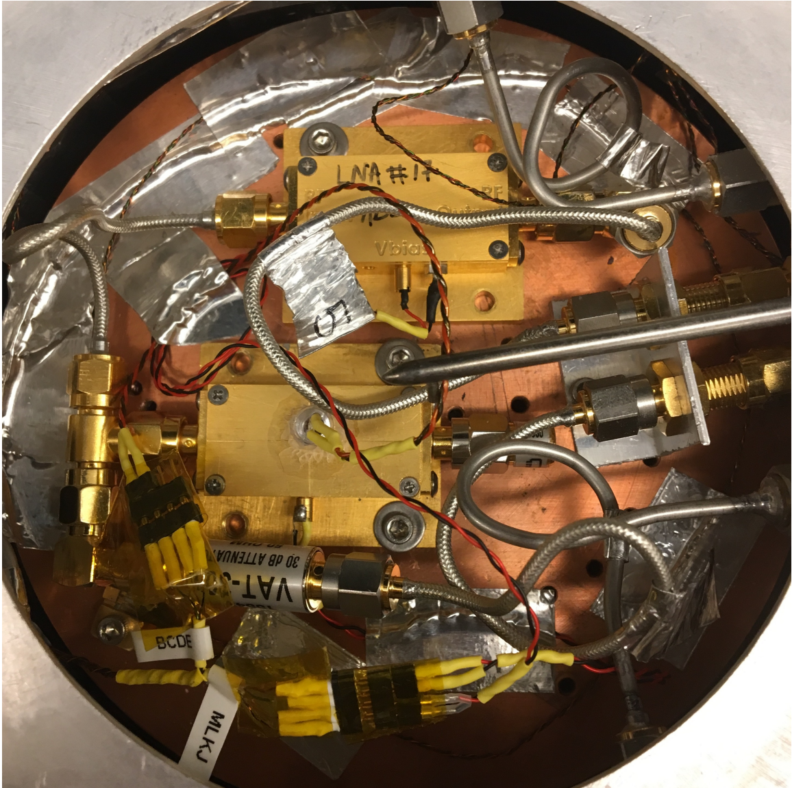
Figure 15: The inside of the liquid helium Infrared Laboratories, Inc. HD-3 cryogenic dewar. The implemented cold 30dB attenuator and ASU cryogenic LNA are connected to the SNRSPD package. A 1300nm central-wavelength LED was situated above the nanowire chip for photon power absorption experiments.
