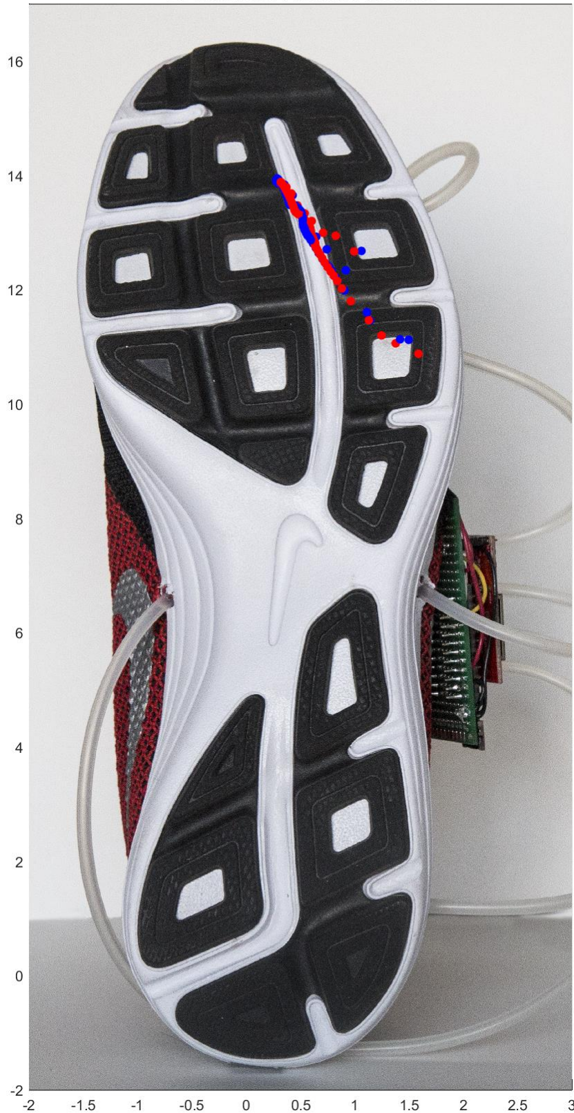
Figure 5.22: Red: Foot force prediction for a single step vs Blue: foot force observations during same step shown as a force trajectory across the bottom of the shoe for stairs.
