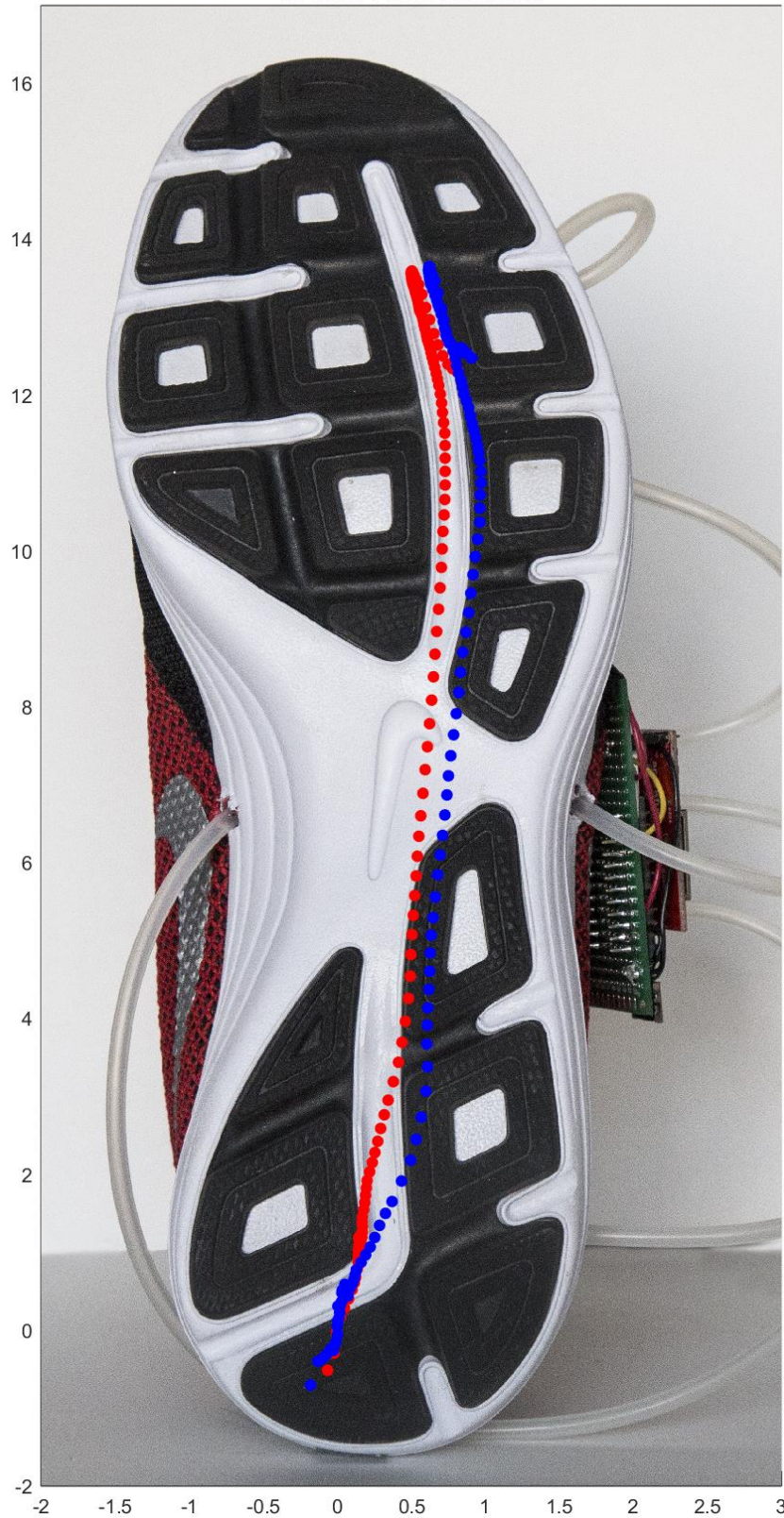
Figure 5.16: Red: Foot force prediction for a single step vs Blue: foot force observations during same step shown as a force trajectory across the bottom of the shoe for level ground walking.
