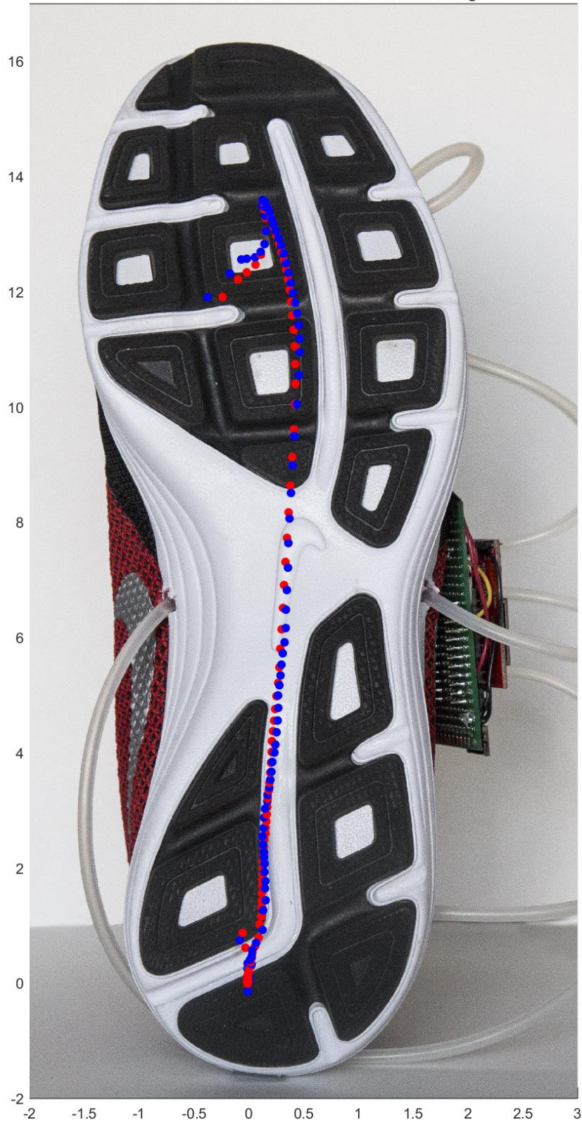
Figure 5.19: Red: Foot force prediction for a single step vs Blue: foot force observations during same step shown as a force trajectory across the bottom of the shoe for inclines.
