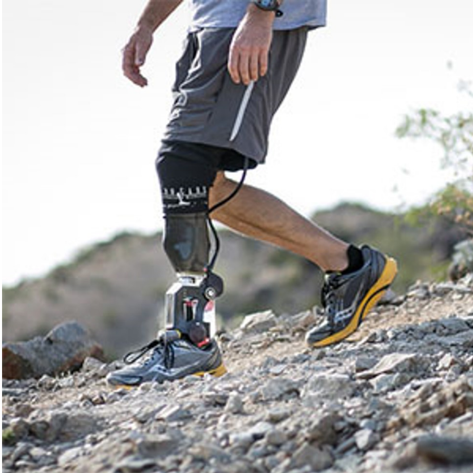
Figure 6.1: SpringActive inc. Odyssey Robotic Ankle.
