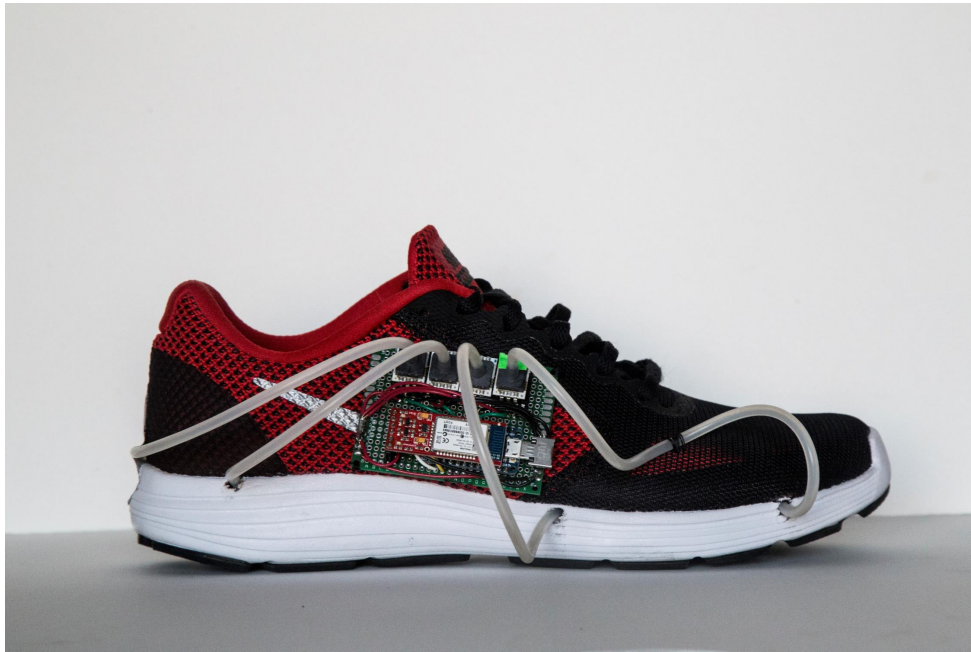
Figure 3.1: Force Sensitive Shoe Platform
