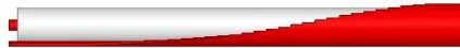
Figure 7.6: Tapered coaxial cable used as a wideband balun to feed the spiral.
