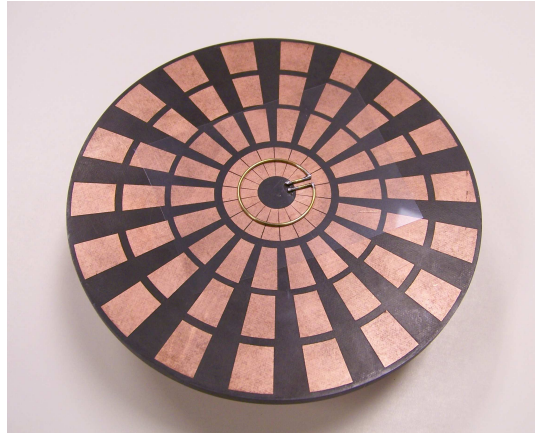
Figure 7.1: Fabricated circular HIS with the loop antenna at a height of 0.01\lambda .
