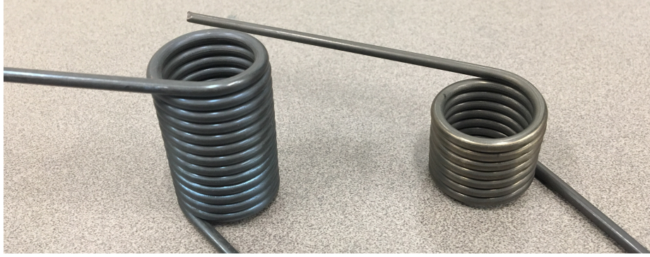
Figure 2.8: Different torsion springs that can be used in the exoskeleton version 2.
