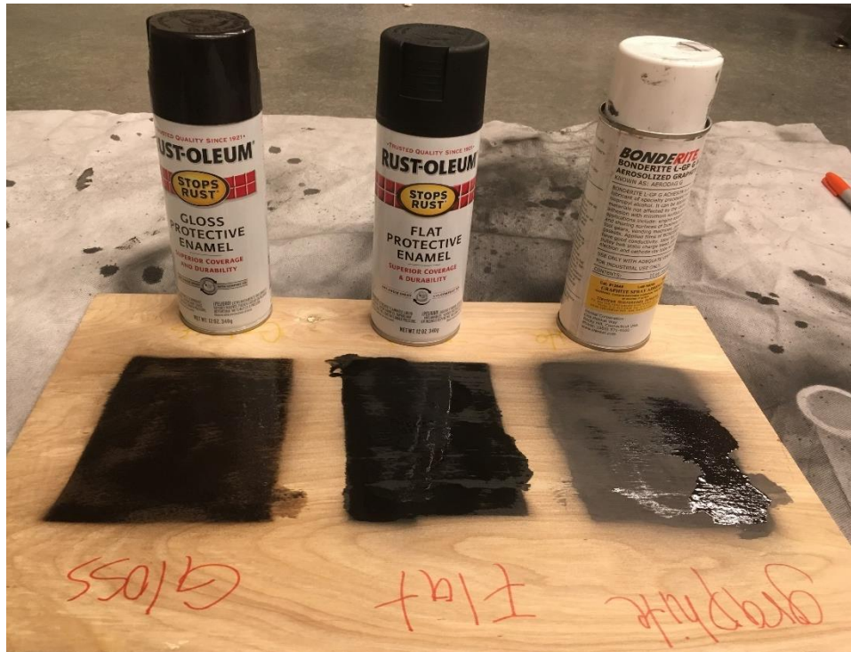
Figure 83. Flat protective enamel by Rust-Oleum black paint was used as a selective absorber due to its high performance under solar radiation
