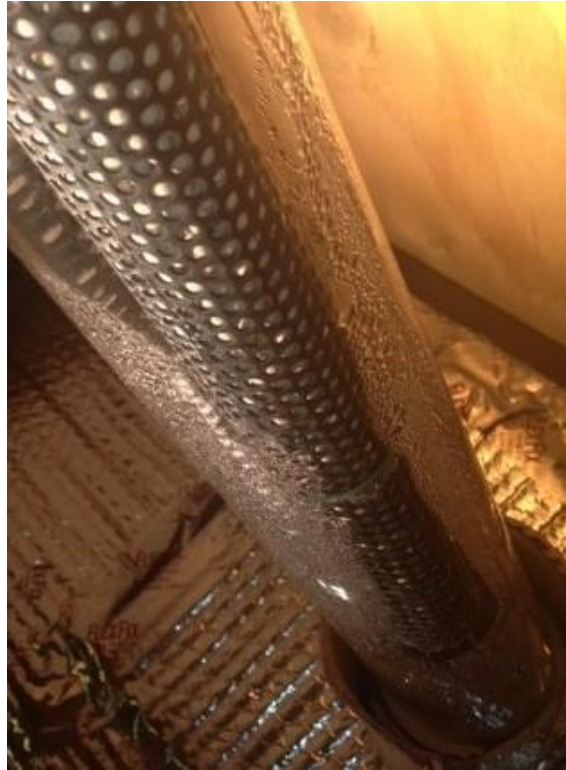
Figure 96. Condensation on the inner glass is one of the major advantages of our evacuated tube adsorption heat pump module
