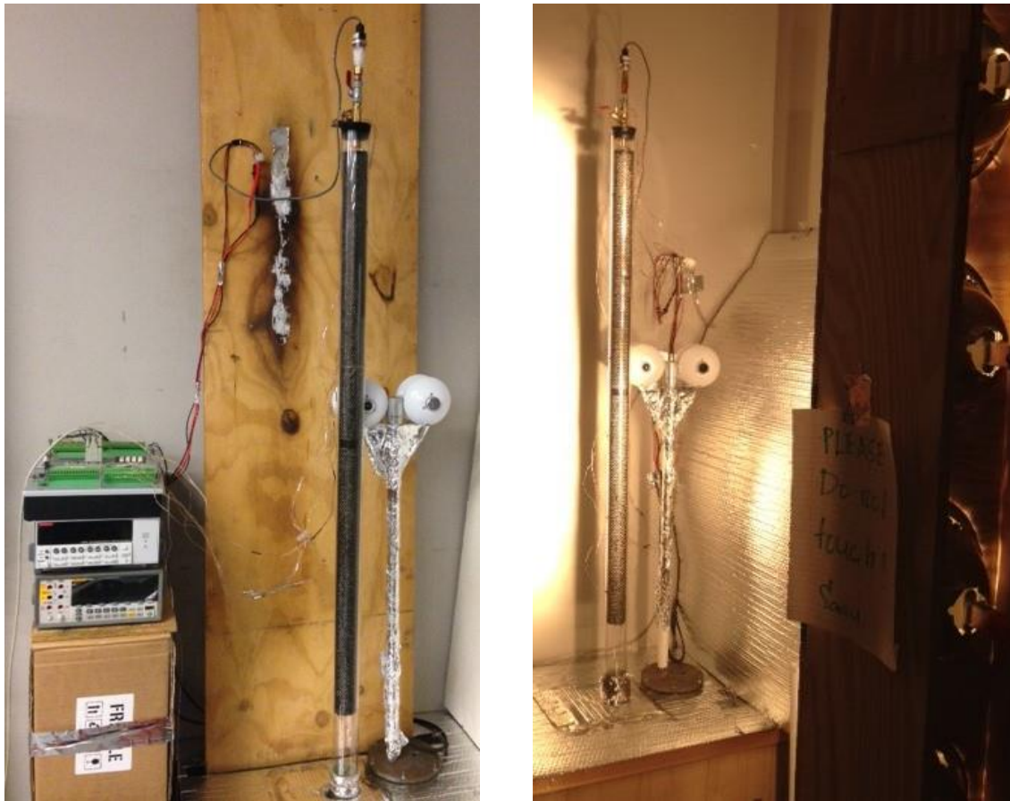
Figure 81. The experimental apparatus of the evacuated tube adsorption heat pump module during adsorption process (left) and desorption process (right)
