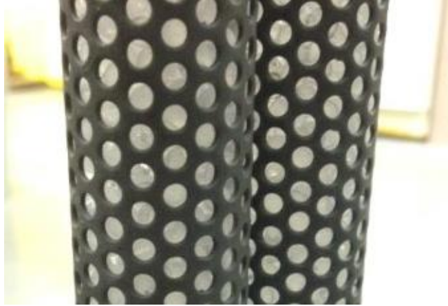
Figure 82. Perforated stainless steel adsorbent bed cage with 3.18 mm diameter holes on 4.76 mm staggered centers (40% open area)
