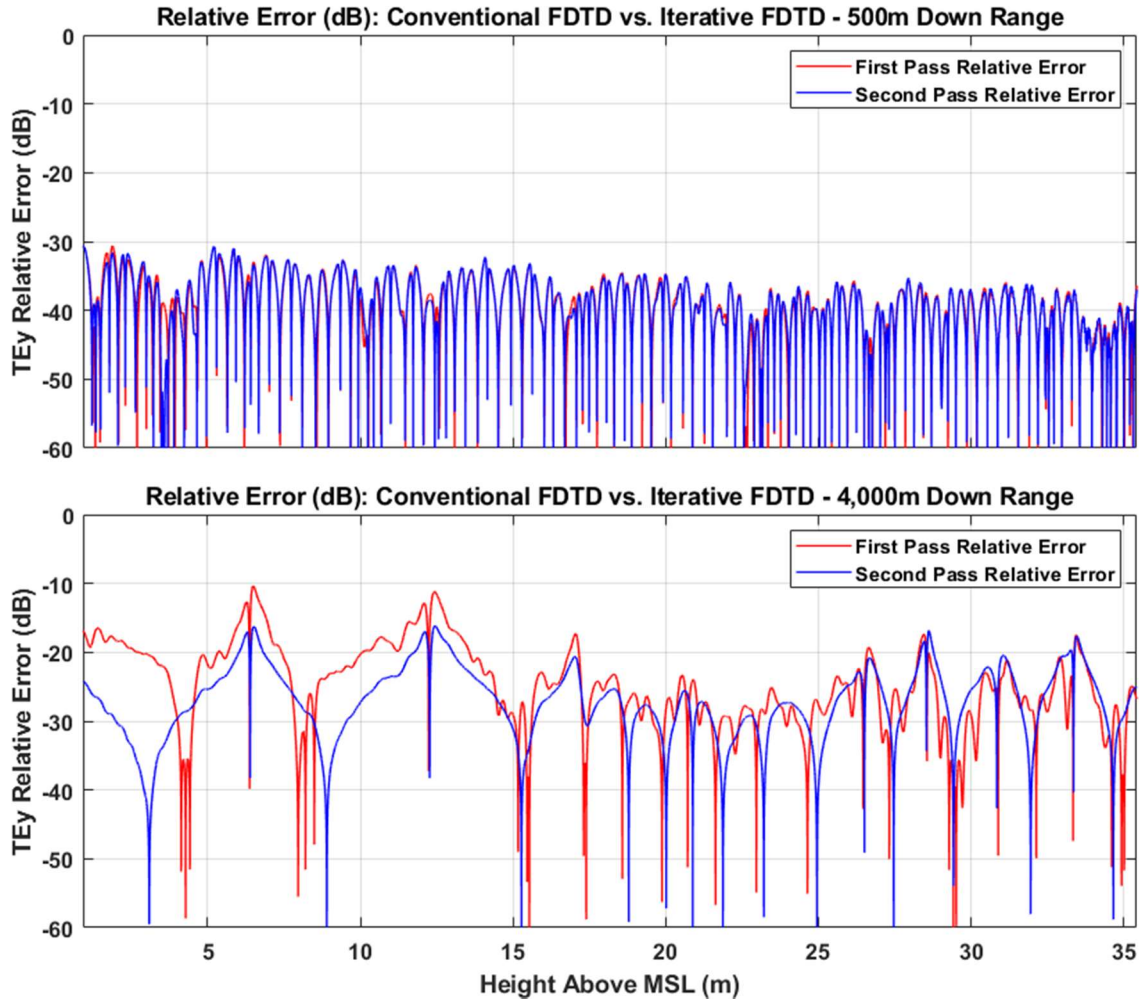
Figure 9.6: Relative error in E_y for the line cut comparisons 500m and 4,000m down range.
