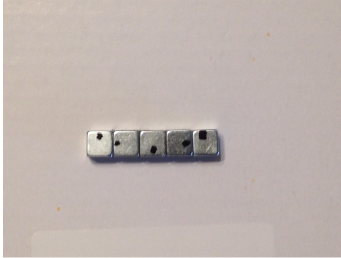
Figure 4.5: Halbach Array Concept with Permanent Magnets
