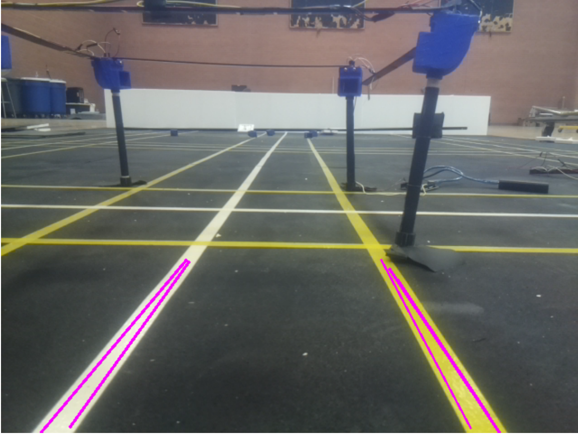
Figure 4.12: Probabilistic Hough transforms detecting the lines on the lane with minimum length of 10 pixels and maximum line gap of 20 pixels
