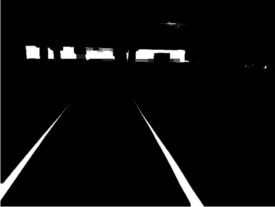
Figure 4.9: Image after eroding with kernel size of 11x11
