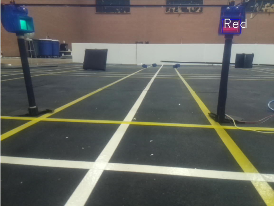
Figure 4.17: Bounding box around red traffic light, the height and the width of the rectangle is used to estimate the distance of the traffic light
