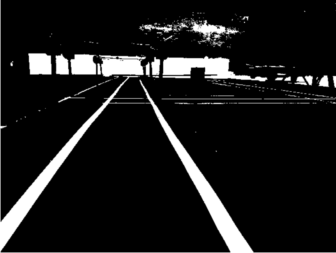
Figure 4.7: The HSV image is masked for pixels with high Value and is represented as a binary image
