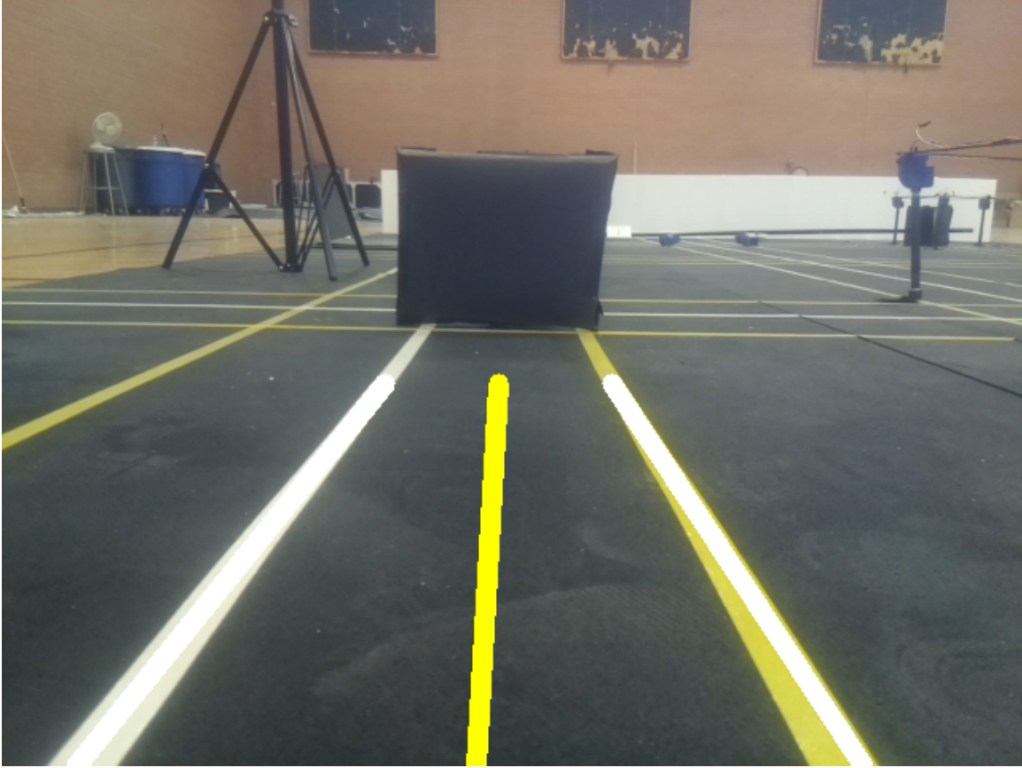
Figure 4.13: The centre of the two lanes is estimated by averaging the left and the right lane pixel positions
