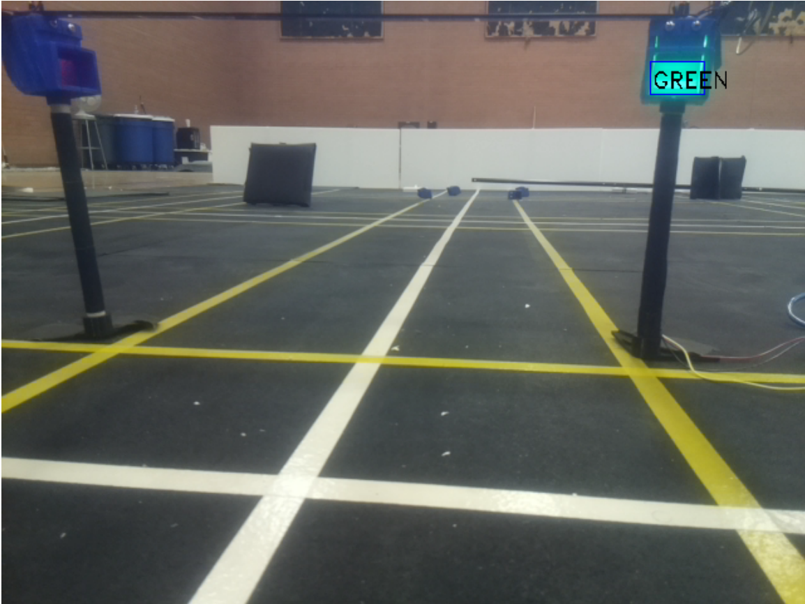
Figure 4.18: Bounding box around green traffic light. The text on the video is used for post analysis
