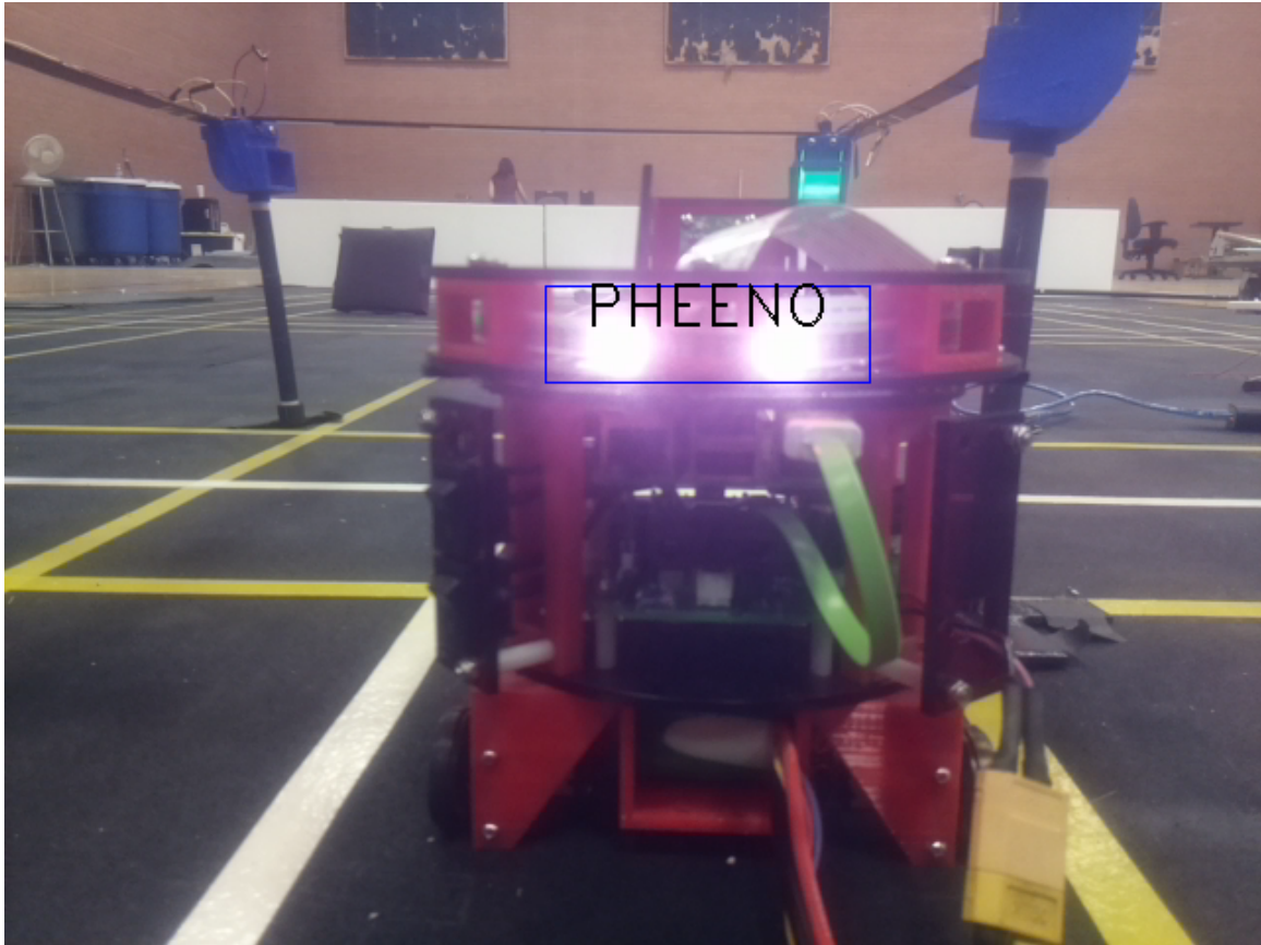
Figure 4.21: Bounding Box around the LED of the robot ahead which is used to estimate the distance of the robot in front
