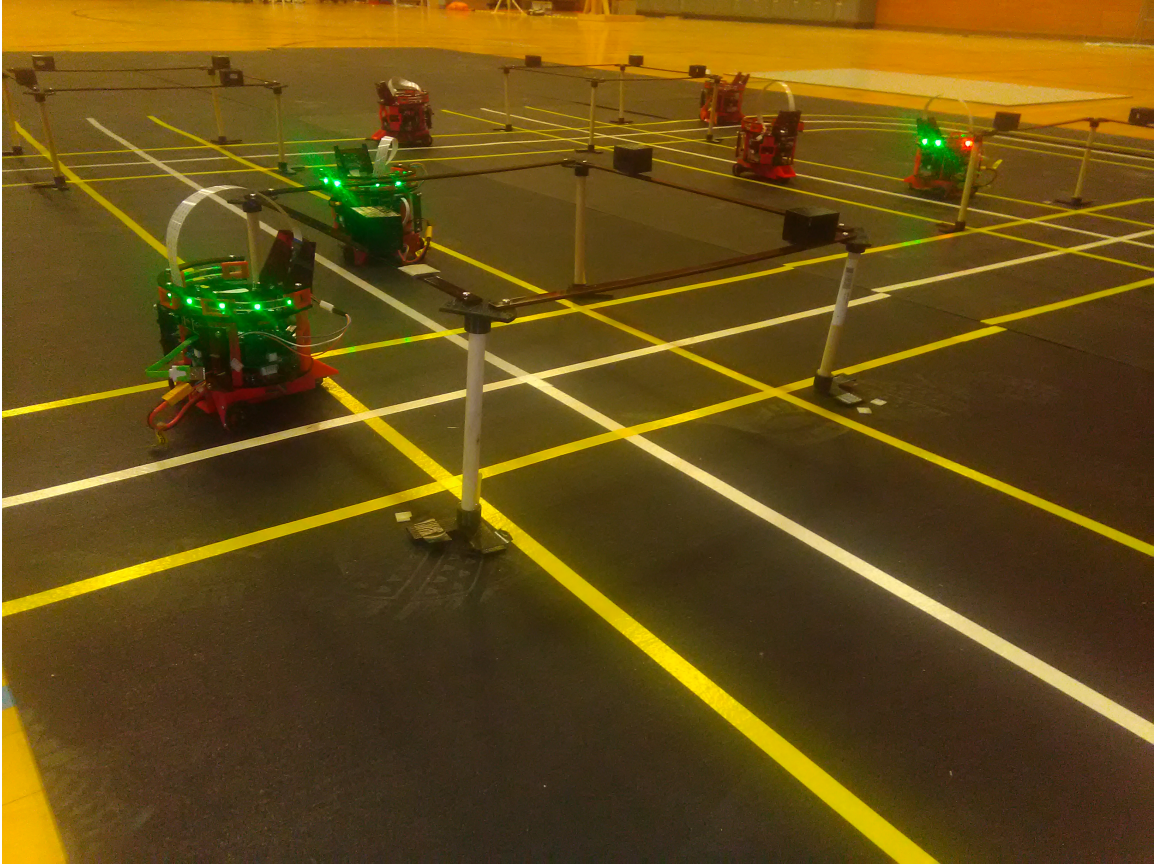
Figure 4.1: Construction of the test bed with the intersection and the traffic lights mounted
