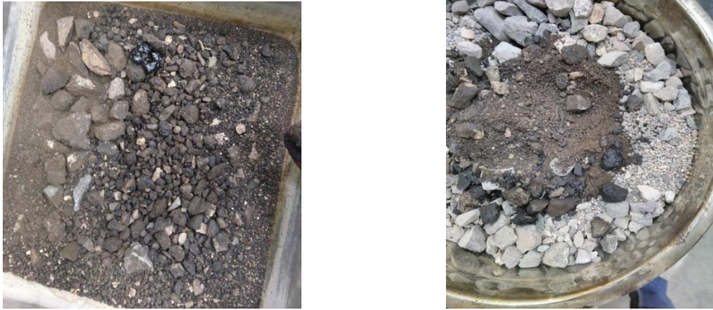
Figure 3.3 Experiments of heating RAP before mixing, left photo case-1, right photo case-2.
