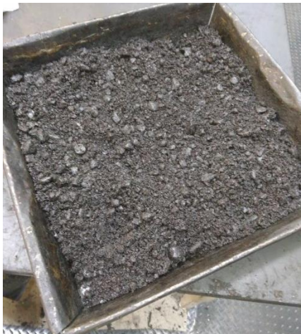
Figure 4.3 Spreading the HMA flat on pan for short term aging
