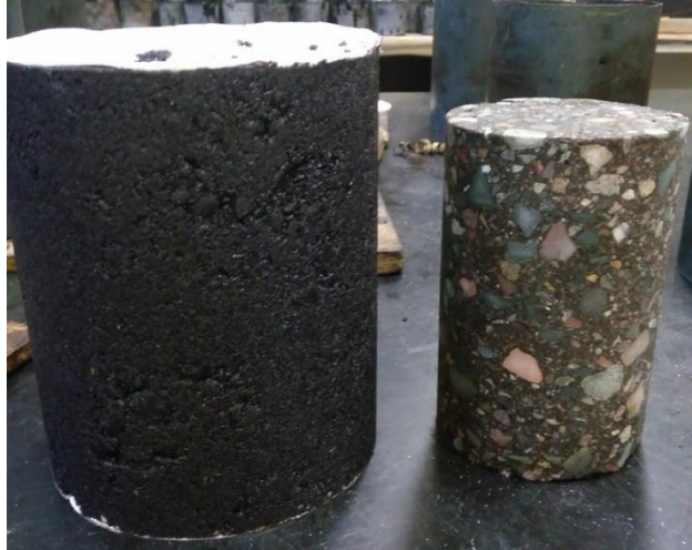
Figure 4.5 Specimen cored and cut from compacted size to required size.
