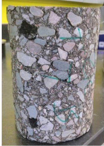
Figure 4.9 Flow number sample after completion of test
