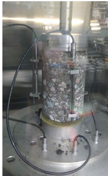
Figure 4.8 Flow number testing for sample
