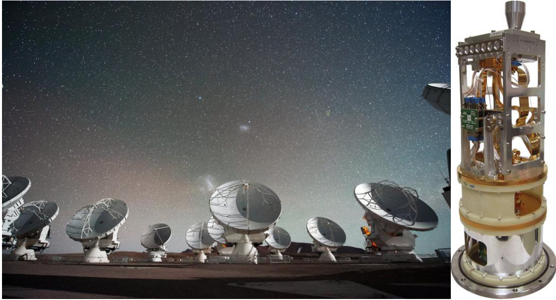
Figure 16: Photographs of ALMA antennas (left) and Band 1 heterodyne receiver (right) covering 35 – 50 GHz from (Malin 2012) and (Morata and Huang 2017), respectively.
