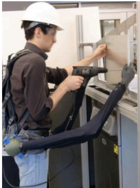
Figure 1: Example of wearable robotic manipulator with two additional arms being used to complete drilling tasks (Llorens-Bonilla, Parietti, and Asada 2012).
