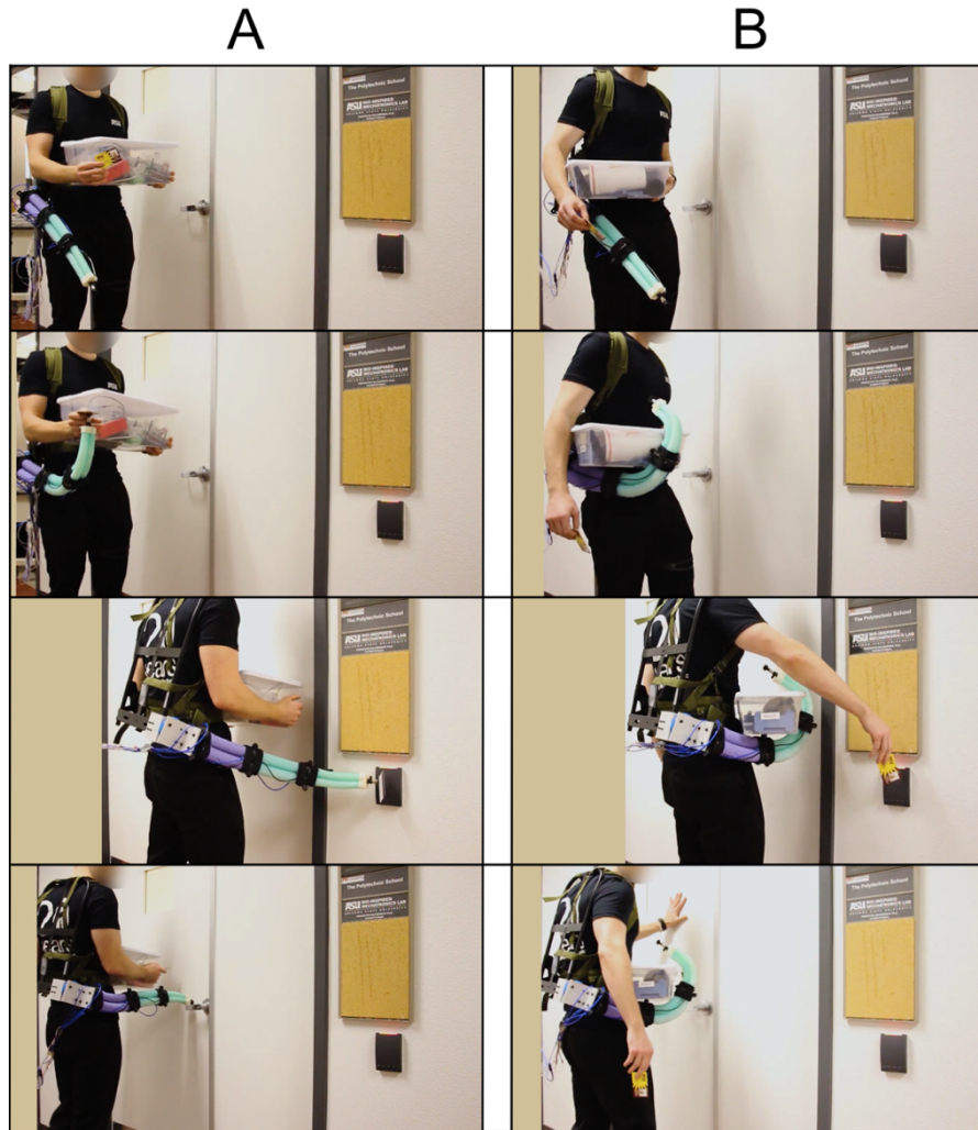
Figure 29: Multi-tasking assistance using the SPL in two ways to accomplish the same task. (A) The user holds a box with both hands while using the limb to scan an access card. The SPL returns the card to the user then pushes the door open. (B) The user holds the box with SPL, using a whole body grasping technique. The hands are free to scan the access card and push the door open.
