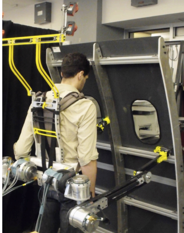
Figure 4: Supernumerary Robotic Limbs assisting a user with the assembly of an aircraft fuselage. The left robotic limb provides contact support while the right limb performs a drilling task (Parietti and Asada 2014).
