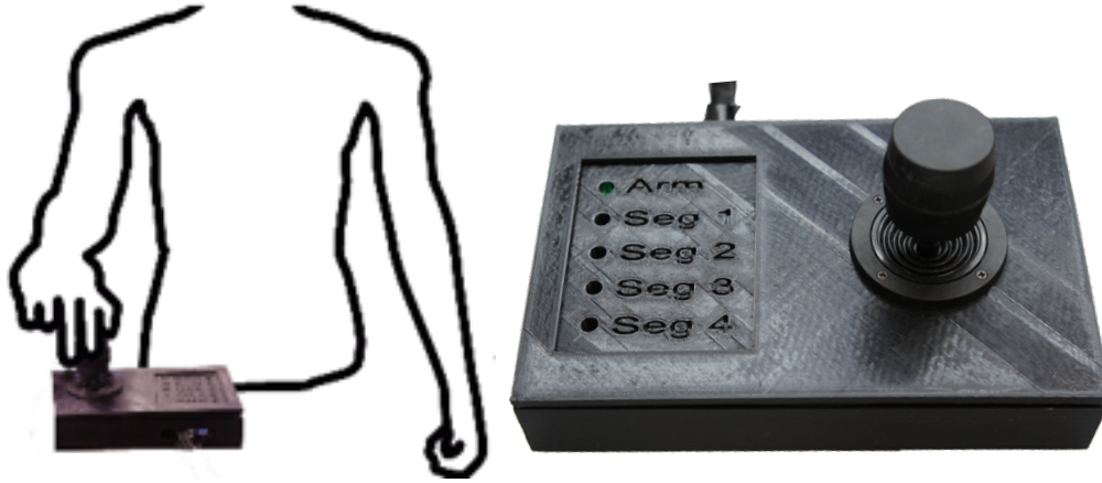
Figure 20: User intent detection via analog joystick is sensed by a change in position along the X, Y, and Z axes. The final box design is on the right.
