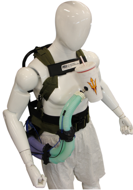
Figure 10: The prototype SPL mounted on a back frame system is a soft, lightweight, wearable robot designed to assist users perform functional tasks.
