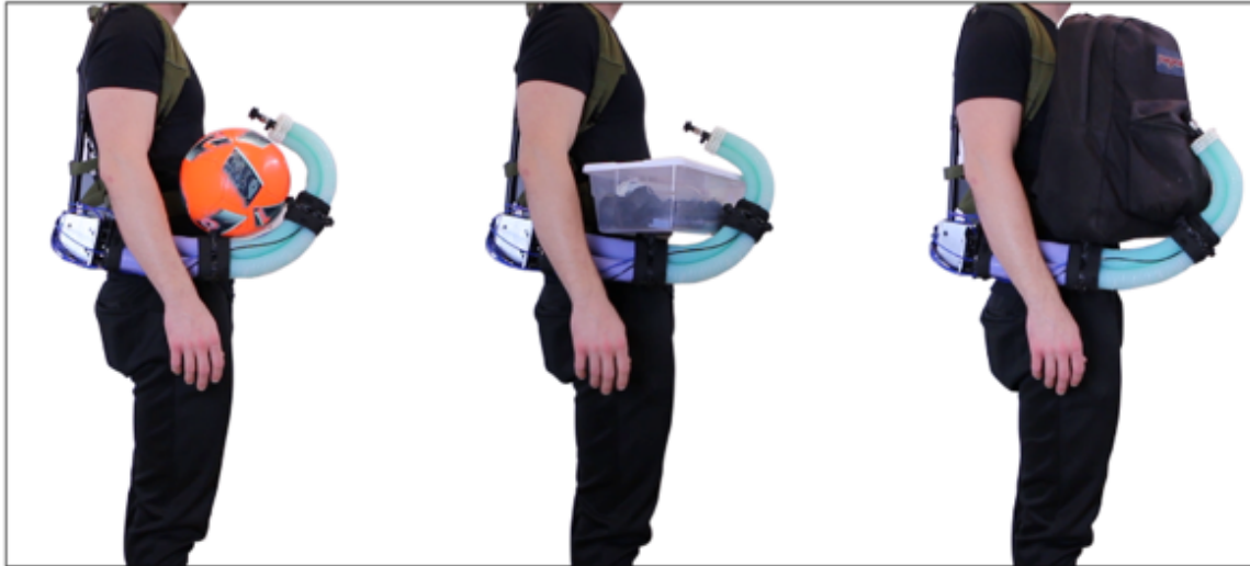
Figure 28: The SPL performing whole arm grasping techniques to carry a ball (0.43kg), a box (0.83kg), and a bag (1.04kg).
