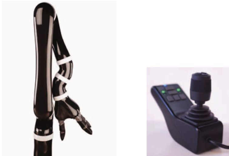
Figure 6: The JACO robotic manipulator and three axis joystick to assist impaired users perform activities of daily living. Movement of the joystick around its three axes positions the robotic arm and grasps objects using the fingers of the manipulator, while buttons on the joystick determine the mode of control (hand positioning, hand orientation, or finger use) (Maheu et al. 2011).
