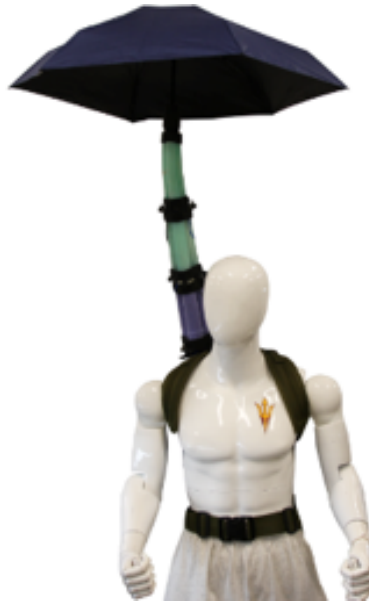
Figure 31: The SPL holding an umbrella (0.25kg) on its distal end to demonstrate potential for overhead manipulation.
