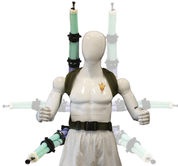
Figure 12: The back frame provides a simple, comfortable means for wearing the SPL. It offers the ability to mount the limb at different positions to work in various task spaces. The opaque limbs are the positions used for testing the SPL in this work, while the translucent limbs provide an example for other possible mounting positions.
