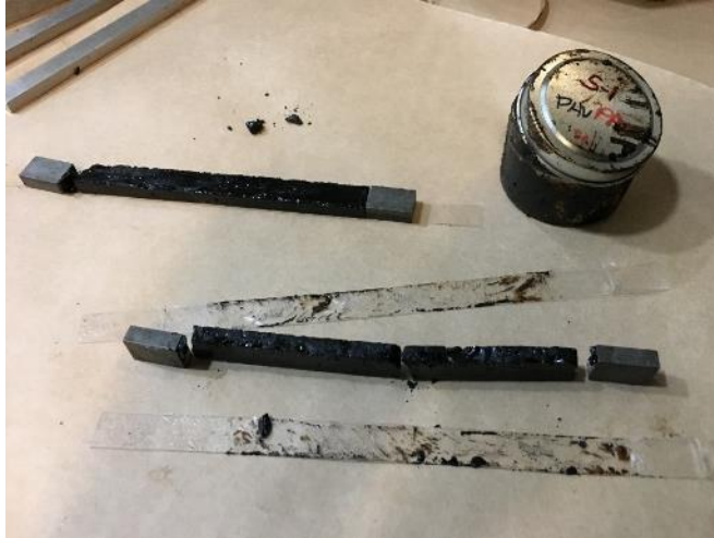
Figure 3-30 Brittle broken BBR beams at the time of demolding.
