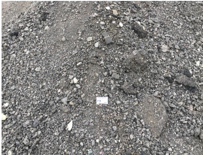
Figure 3-9 Detail of RAP sample S-3.
