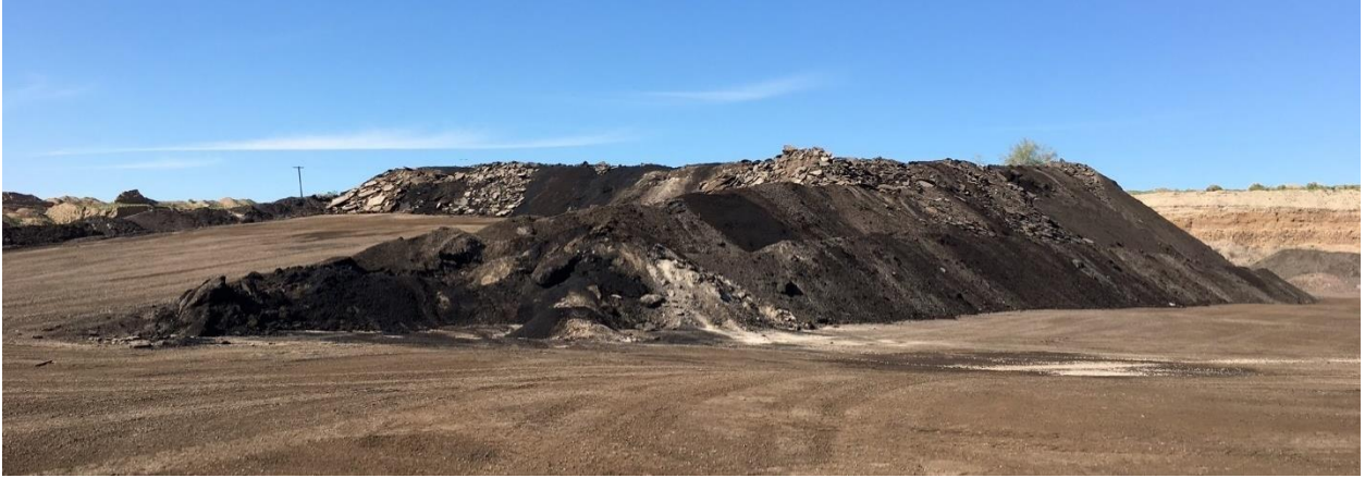
Figure 3-13 Stockpile of RAP millings from Southwest Asphalt of El Mirage Plant
