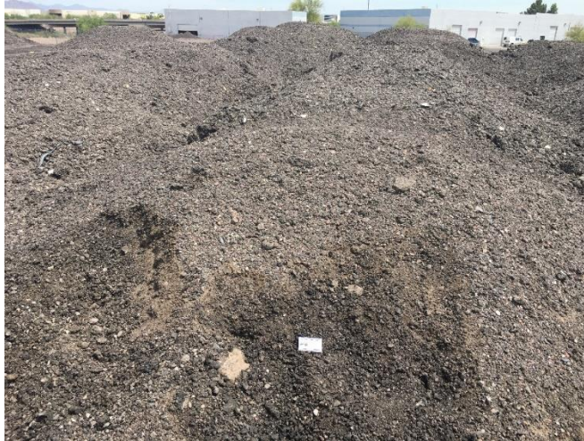
Figure 3-8 Detail of RAP sample S-2
