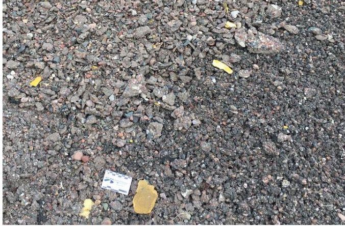
Figure 3-2 Typical unprocessed millings of RAP material (card in lower left corner is approximately 3 inches long and 2 inches wide)
