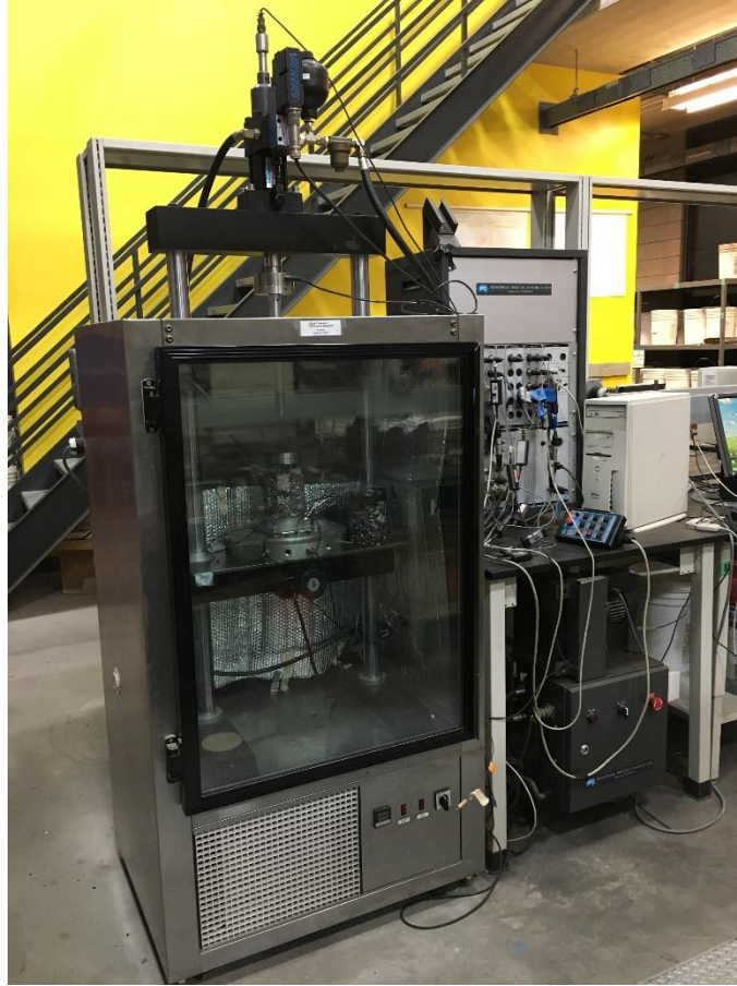
Figure 5-2 Universal testing machine to perform Flow Number Test
