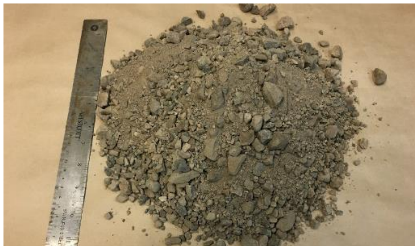
Figure 3-24 Extracted aggregates from Southwest Asphalt plant.
