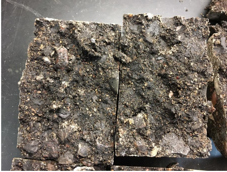
Specimen after split test showing a little striping.
