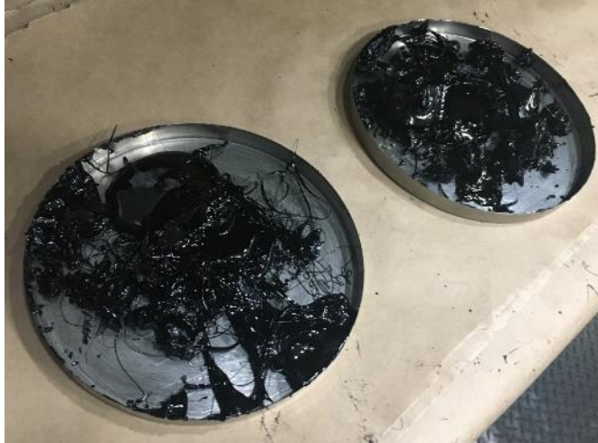
Figure 3-28 Extracted binder poured into PAV pans prior to aging.
