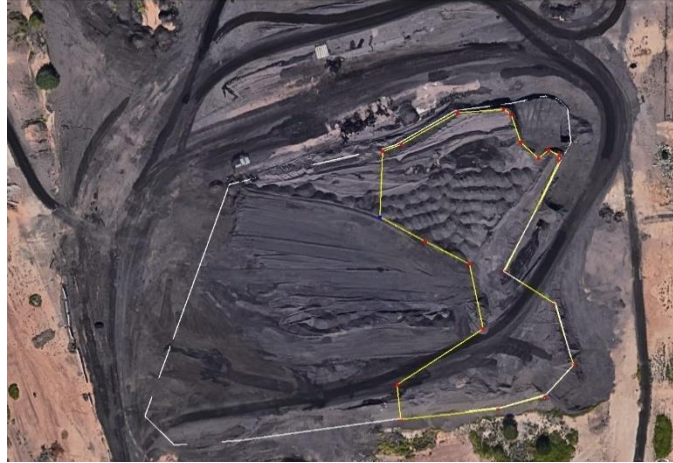
Figure 3-5 Areas for RAP volume estimation of the main stockpile
