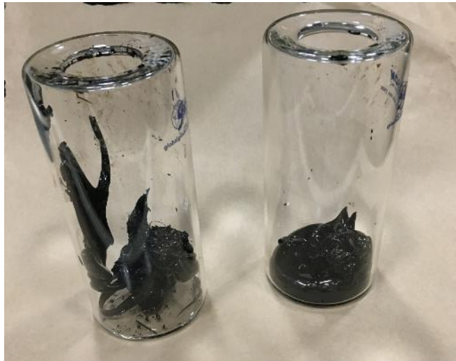
Figure 3-27 Extracted binder poured into RTFO bottles prior to aging.
