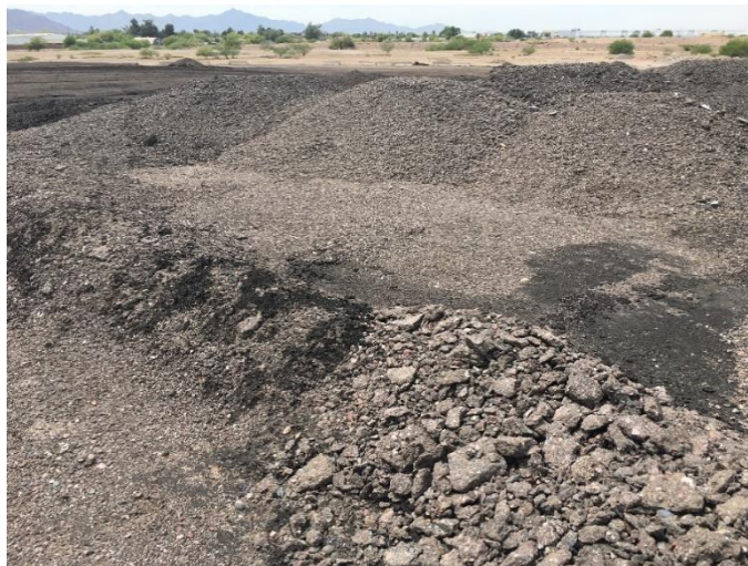
Figure 3-4 Small piles of RAP millings over the top of the main RAP stockpile
