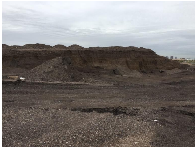
Figure 3-1 General view of a single RAP stockpile
