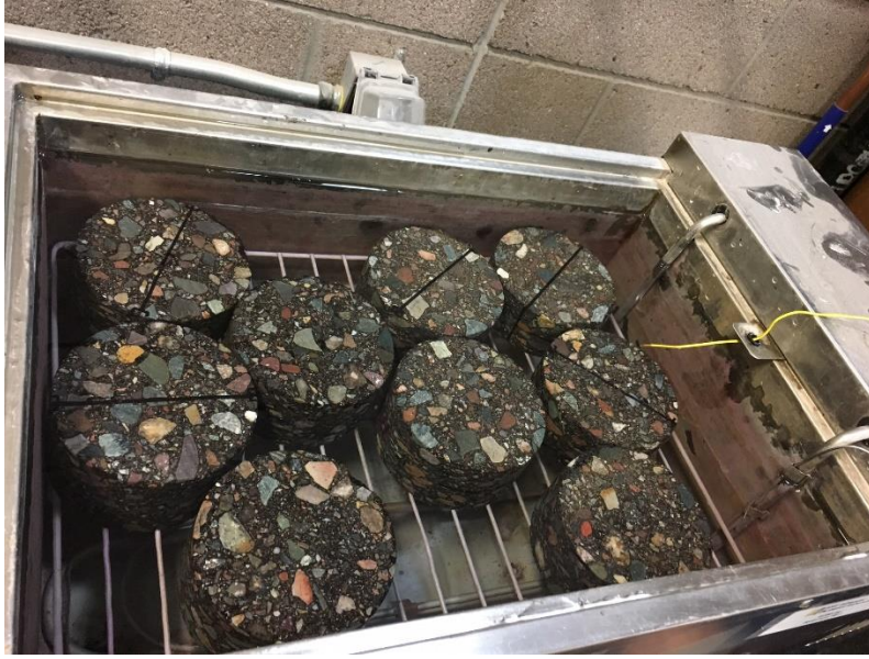
Water bath of conditioned specimens at 140°F (60°C) for 24 hrs.
