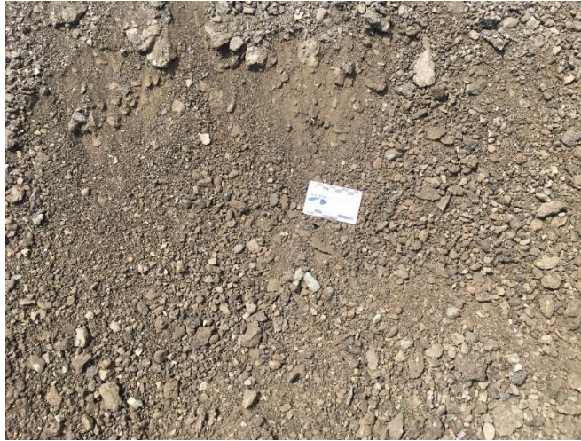
Figure 3-7 Detail of RAP sample S-1
