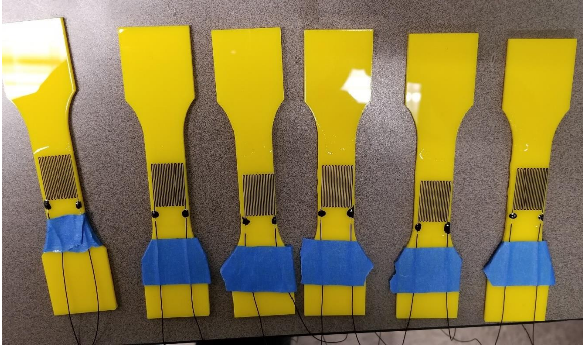
Figure 34: Strain gauges printed on acrylic dog bones
