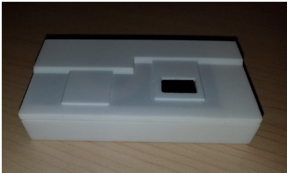
Figure 47. The Assembled Recharging Base Unit for either Inductive Recharging or Direct Recharging
