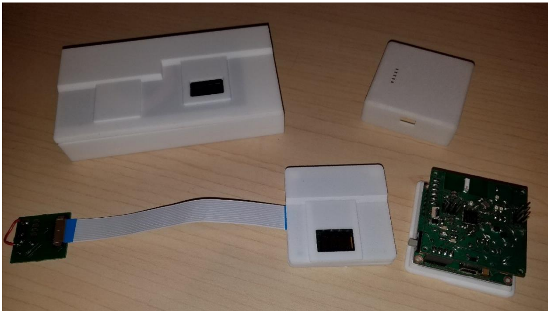
Figure 28. Overview of the Three Units (Recharging Base, Mounting Base, and Transmitter) That Make Up the Complete Wireless Strain Transmitter System
