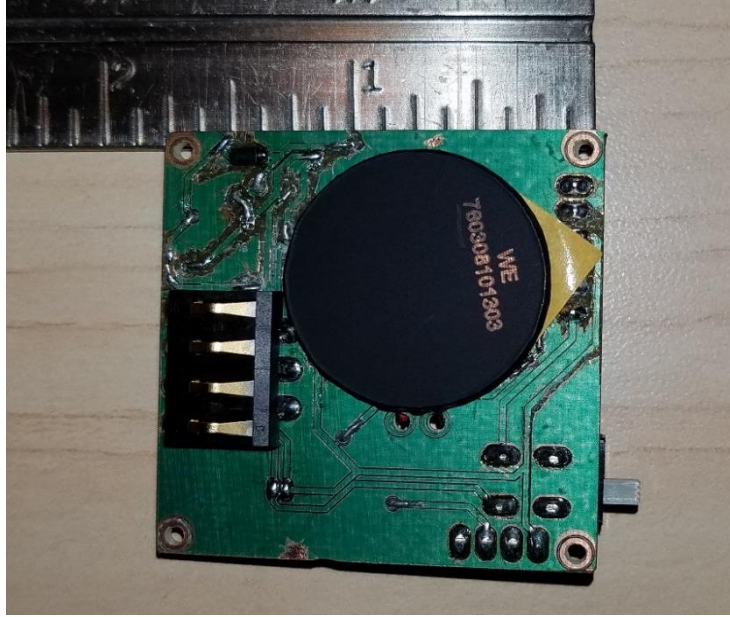
Figure 31. Bottom Face of the Assembled PCB for the Receiving Inductive Battery Recharging
