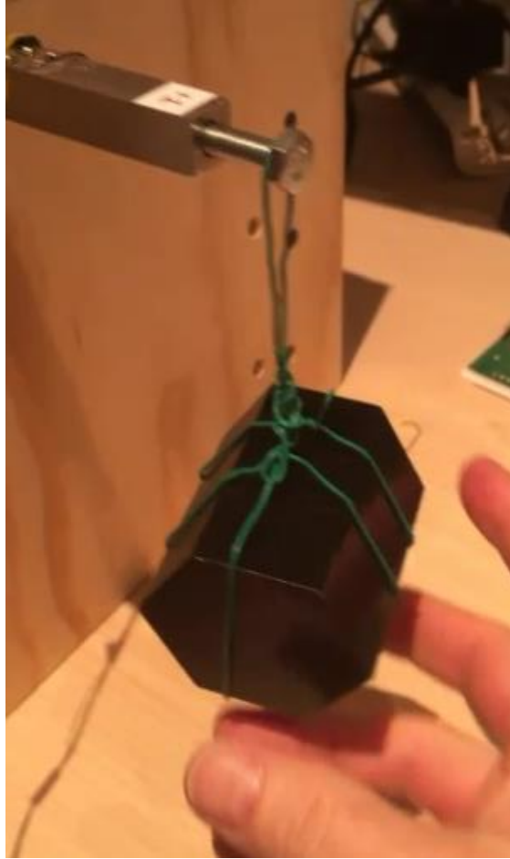
Figure 56. Clipped Image from the Demo Video of a Known Weight of 1003 Grams Being Applied to Full-Bridge Strain Gage Setup on an Aluminum Rod
