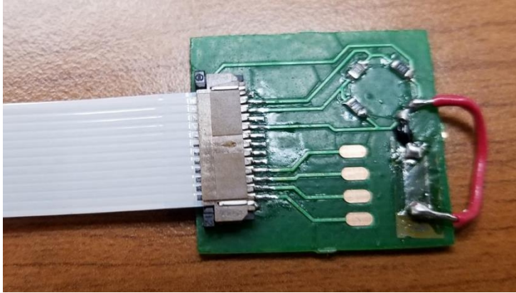
Figure 46. Strain Gage Interface PCB Board Where a Strain Gage can be Connected Up to the System
