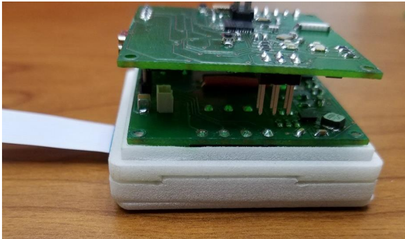
Figure 44. Close Up of the Mounting Base Fitted with the Transmitter Unit in an Inductive Recharging Configuration with the Transmitter Top Case Piece Removed
