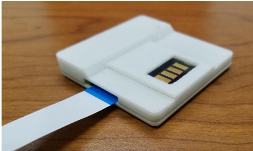
Figure 43. The Assembled Mounting Base in the 3D Printed Case
