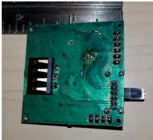
Figure 35. Bottom Face of the Assembled Direct Power Battery Recharging
