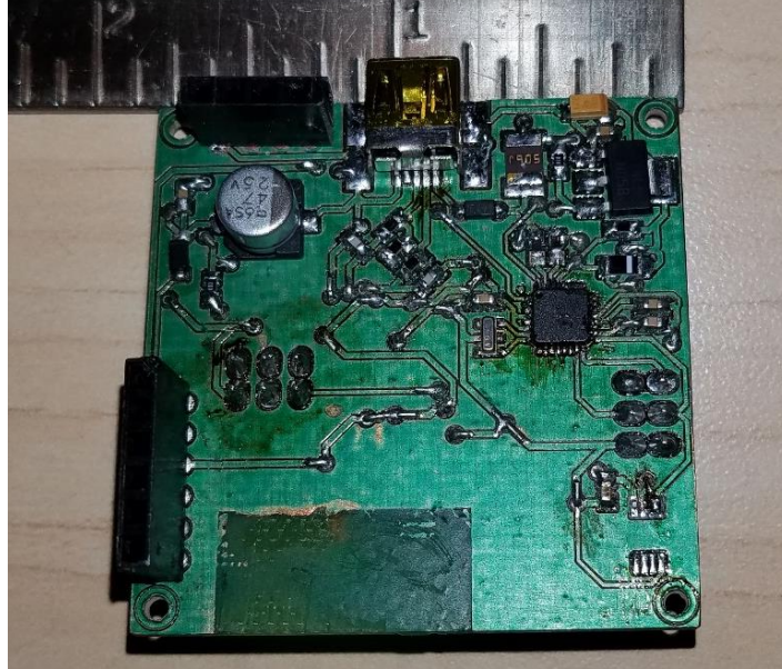
Figure 40. Microcontroller Face of the Assembled PCB for the Microcontroller and Bluetooth Layer
