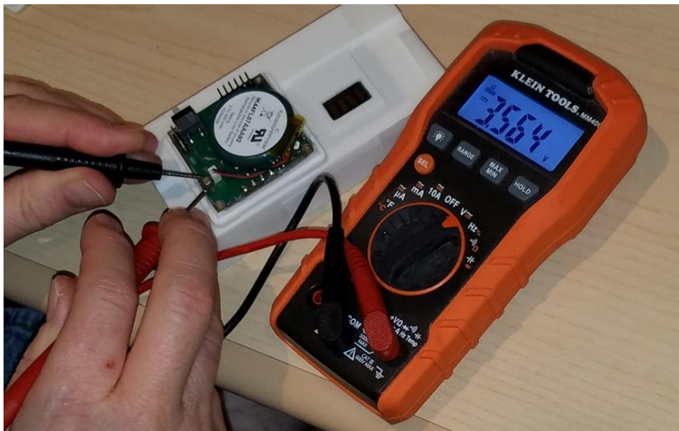
Figure 52. Validation Testing of the Battery Power for Inductive Battery Recharging
