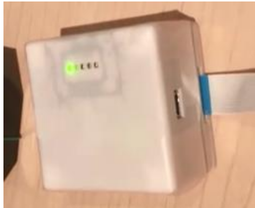
Figure 53. Clipped Image from the Demo Video of the Power Indicator LED Being On After System Was Switched On
