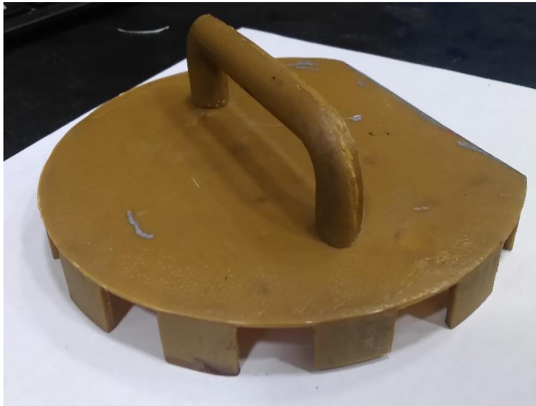
Figure 41: Cutting Template for the Hamburg Wheel Test Samples
