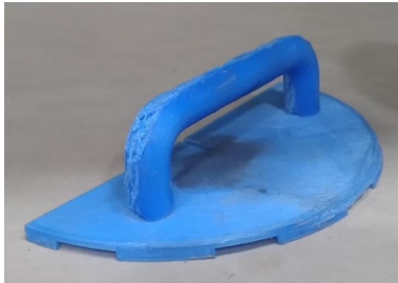
Figure 39: Cutting Template for SCB Samples
