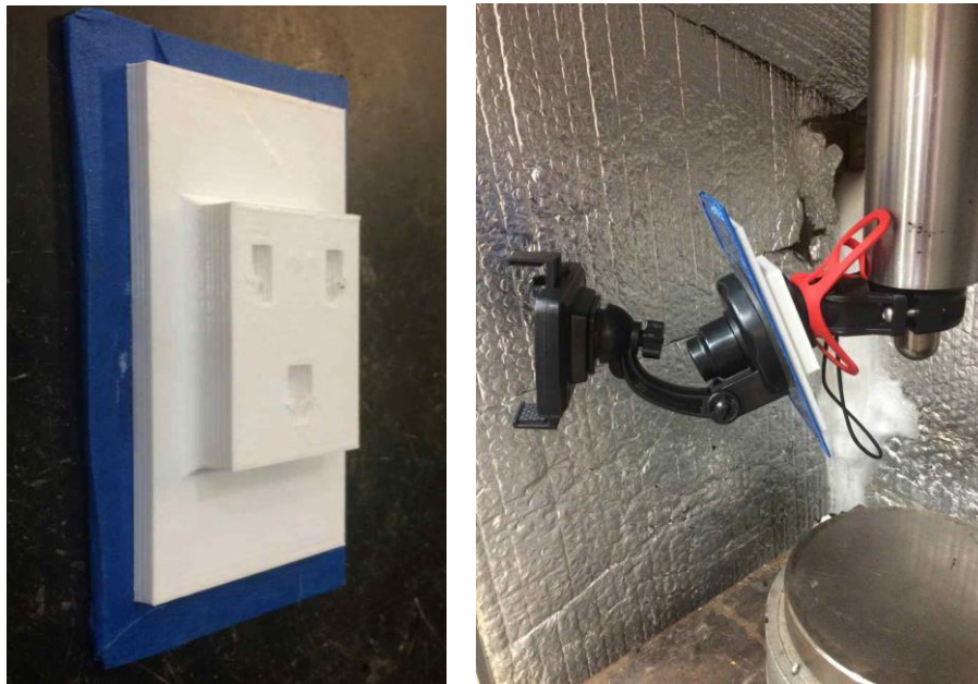
Figure 43: Cell Phone Mount for IRI Measurements
