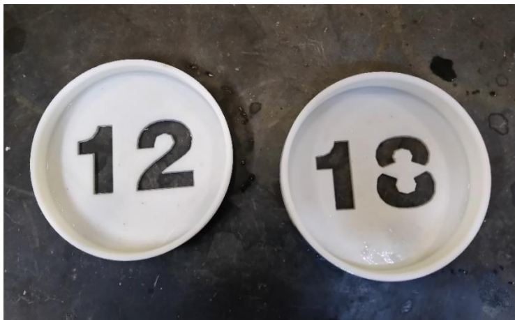
Figure 37: End Sawing Jigs for Cored Gyrotory Samples
