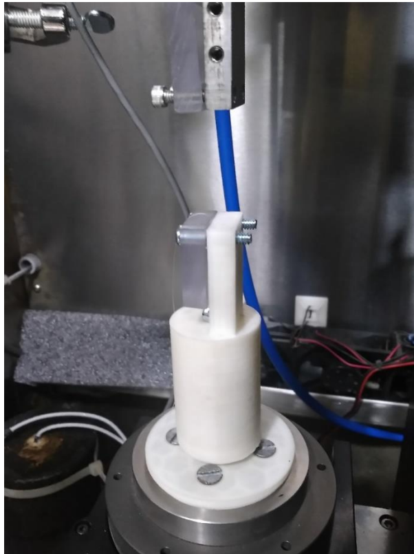
Figure 40: Fiber Pull-out Testing Apparatus
