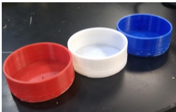
Figure 45: Binder Cups for Fiber Pull-out Test
