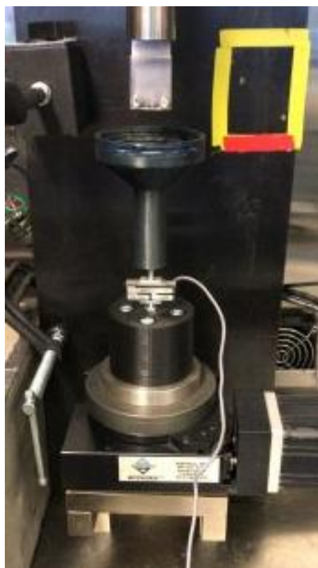
Figure 46: Binder Cup Mount and Load Cell Spacer for Fiber Pull-out Test
