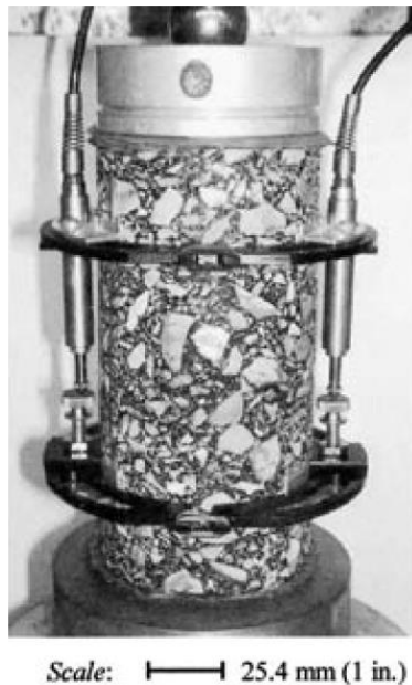
Figure 4: Split Spring Collars Used to Attach LVDTs To Asphalt Concrete Samples [5].
