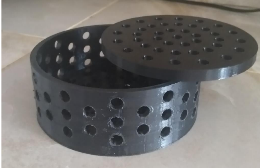
Figure 47. Confinement Device for Circular Test Samples
