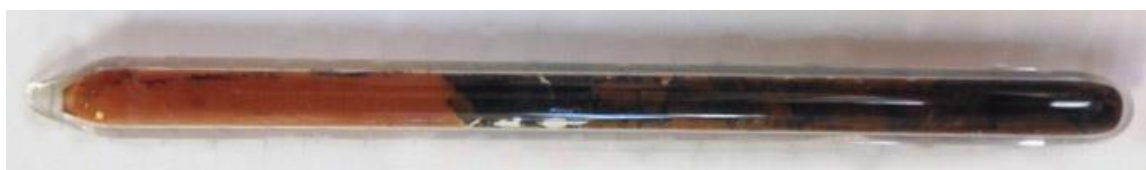
Figure 57. Fused silica tube containing the post-reaction mixture of myo -inositol in water alone (250°C, 48h). The reaction started out as a clear, colorless, solution.
