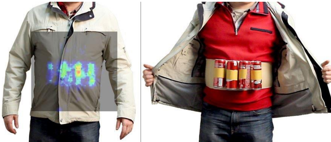
Figure 1-5 A THz image of a dummy explosives belt (Courtesy of TeraSense Development Labs).
