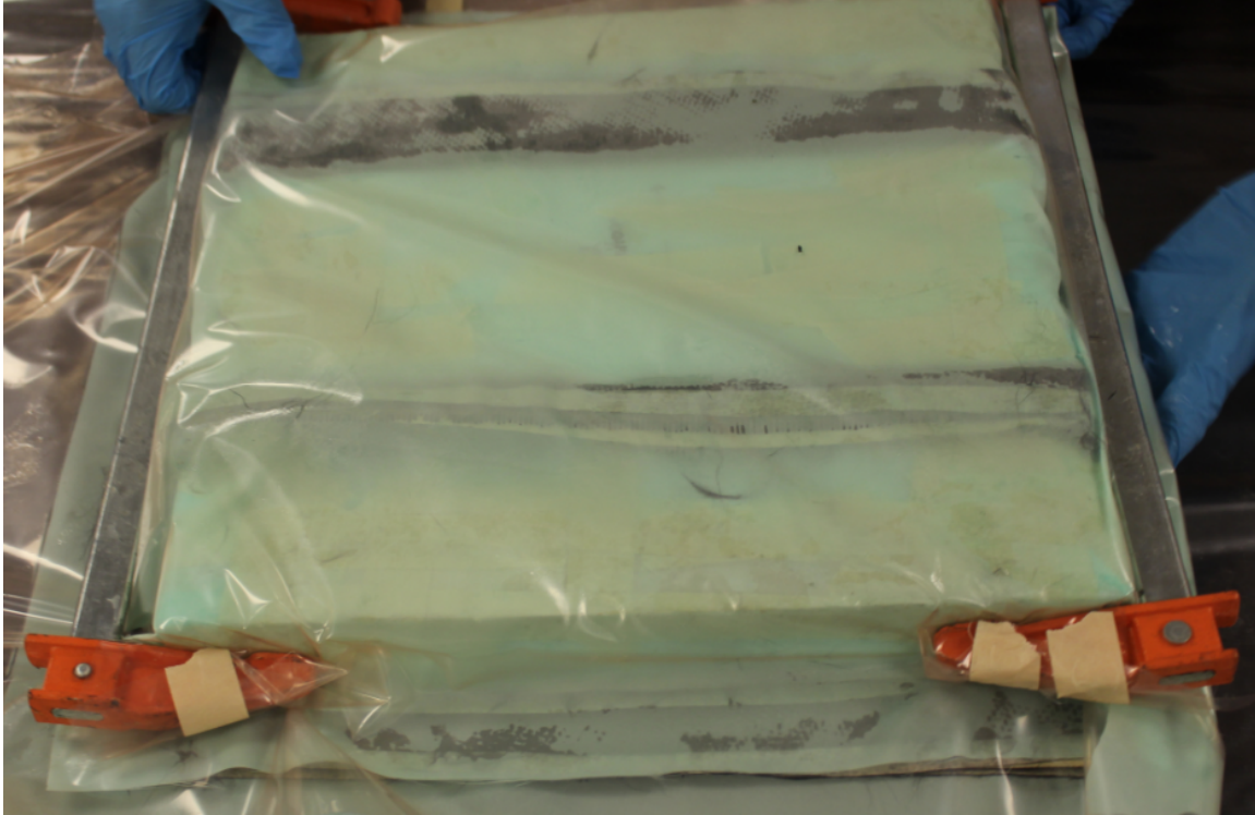
Figure 7.3. Clamped pre-cure stiffened panel within mold
