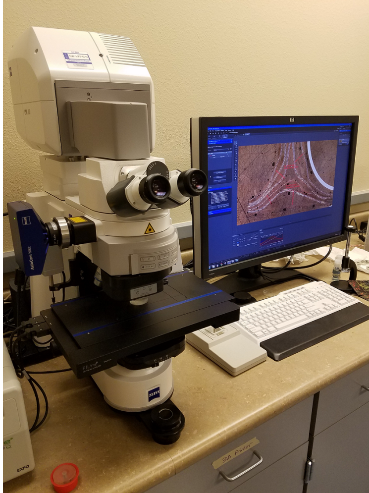
Figure 7.6. Zeiss LSM 780 confocal microscope used for microscopy of the T-joint specimens
