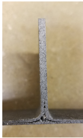
Figure 7.10. Speckle pattern on the face of the T-joint
