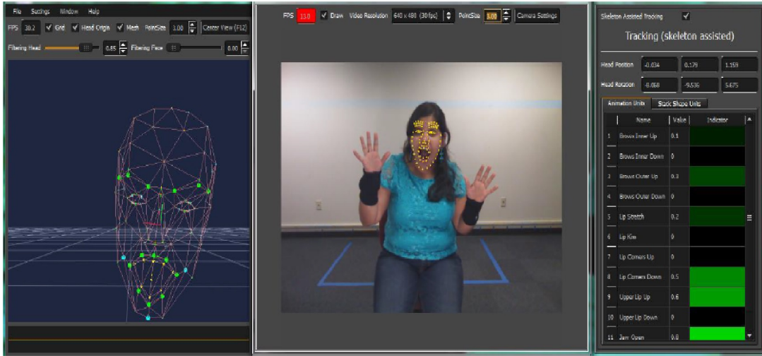
Figure 4.2: Snapshot of a Subject Portraying Emotion, Surprise. Left: 3D Face-Mesh Corresponding to the Emotion. Middle: Brekel Kinect Pro Face Tracking Animation and Shape Units Shown as Yellow Dots Over the Subject's Face. Right: Tracking Indicator Showing Presence or Absence of Animation Units at Each Instant. Best Viewed in Color, Source: Ranganathan et al. (2016a)
