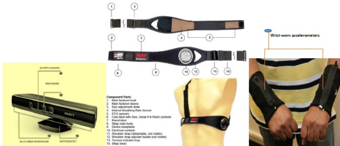
Figure 4.1: Equipment Used for Data Capture. Left: Microsoft Kinect for Windows Sensor With Labeled Components. Middle: Zephyr BioHarness With Labeled Component Parts. Right: Wrist-Worn Accelerometers. Best Viewed in Color
