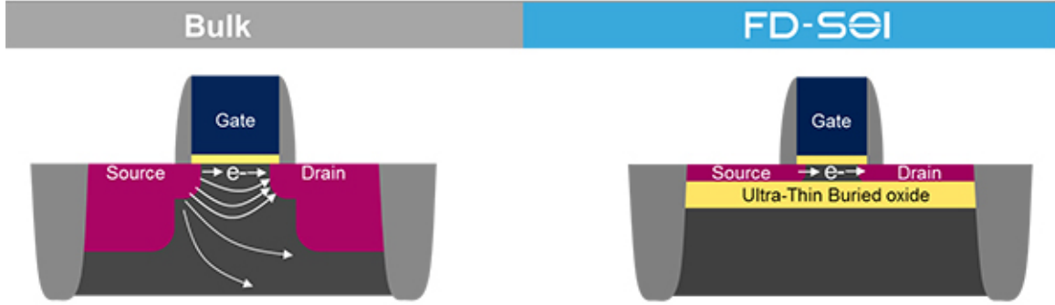
Figure 4.2: Bulk vs FD-SOI technology STMicroelectronics (2018).
