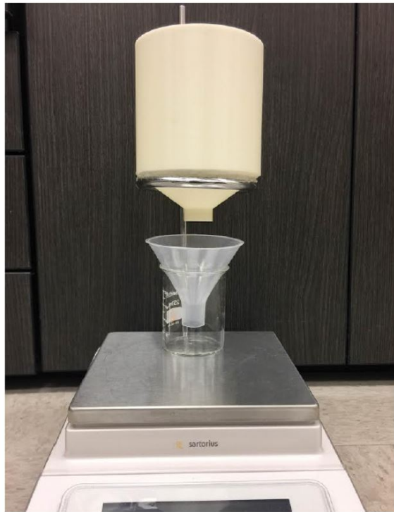
Figure 5: 3D printed hopper used to conduct the experiment for polydispersity implementation validation.
