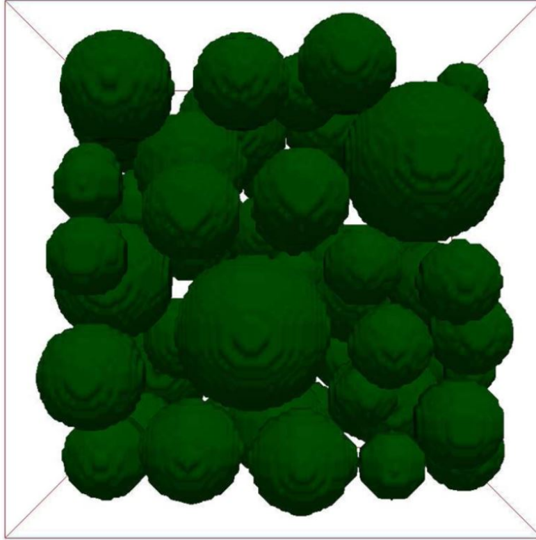
Figure 22: A SiC-particle reinforced Al-matrix composite material with final particle volume fraction \phi = 0.31 . Only the particle is shown and the matrix is transparent. The linear size of the system is 200\mu m . The whole system is digitized into 100 by 100 by 100 voxels.
