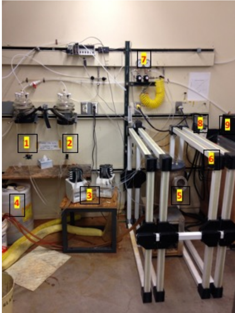
Figure 2.2: Experimental set up for spin spray deposition (SSD)
