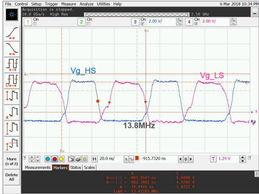
Figure 54: High side and Low side Switching Signals at 13.8MHz
