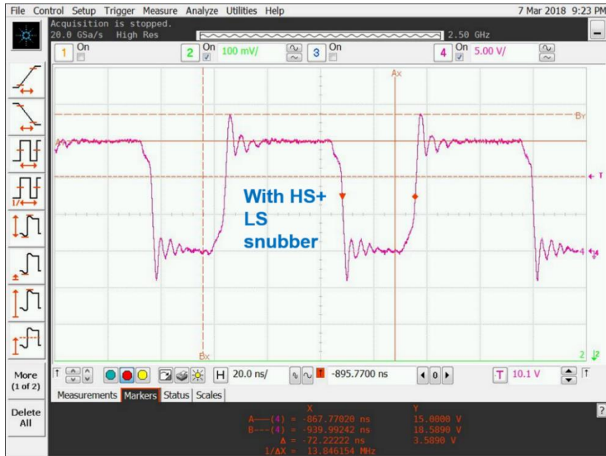
Figure 55: Effect of Snubber on the Switch Node for Ringing upto 3.58\text{V} at 15\text{V} Input Supply
