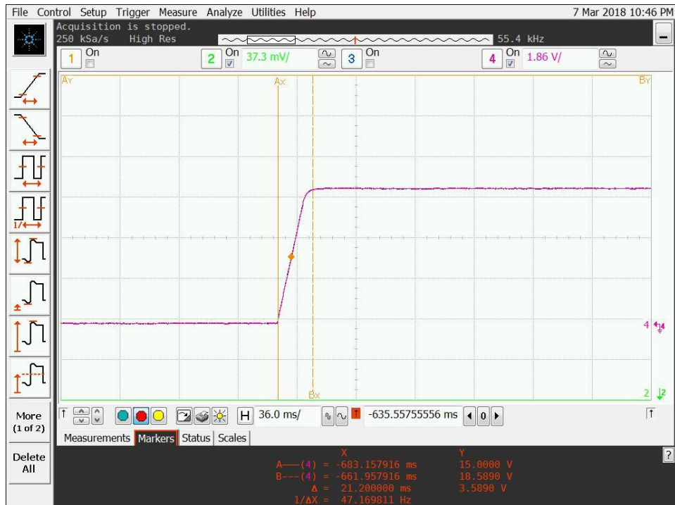
Figure 61: Vout Settling Time as 21.2ms During Start-Up in Open Loop
