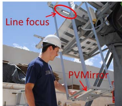
Fig. 6. Photograph of an outdoor test of a PVMirror. The PVMirror is mounted on the tracker and a clear line of visible light is produced at the focus, indicating that the PVMirror performs as a concentrating optic.
