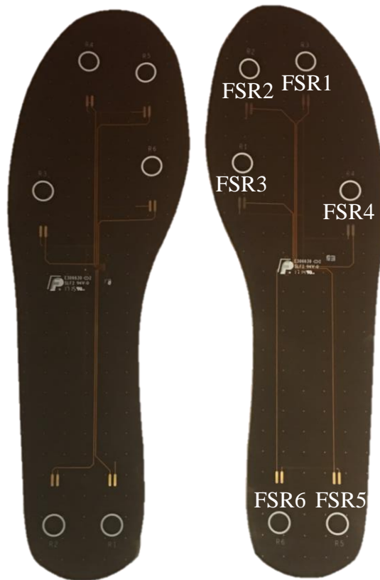
Figure 7: Fabricated insoles with FSR's location
