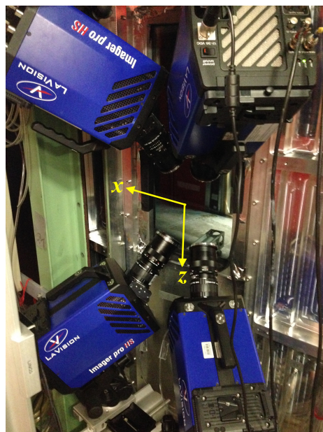
Figure 5.17: Camera configuration of the tomographic TBL measurement.
