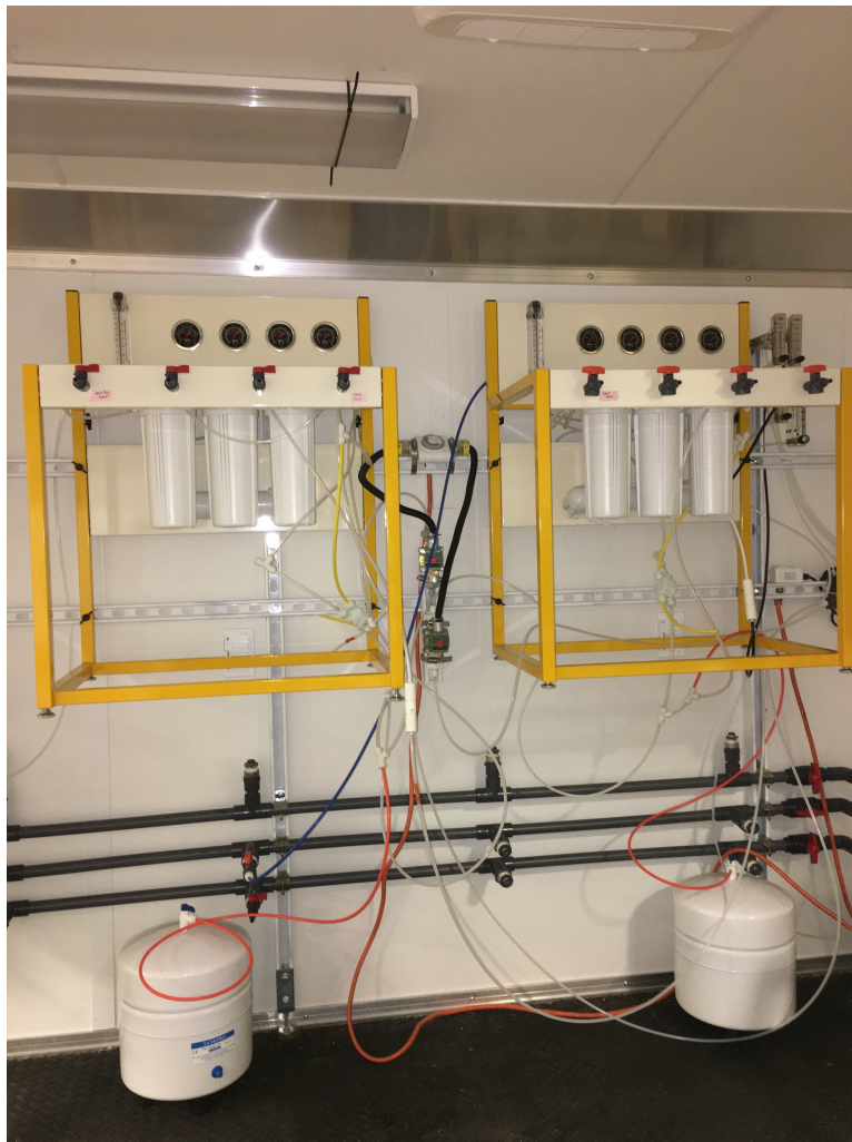
Figure 2.7: Two POU Units with Water Storage Tanks and Solenoid Valves with Timer in Mobile NEWT Testbed (Unit 1 right, Unit 2 left)
