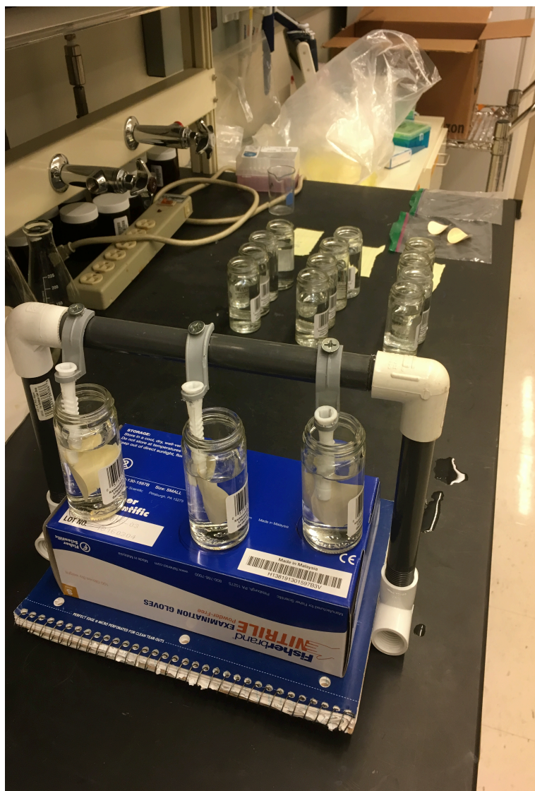
Figure 2.2: Static Leaching Test Configuration After Commencement
