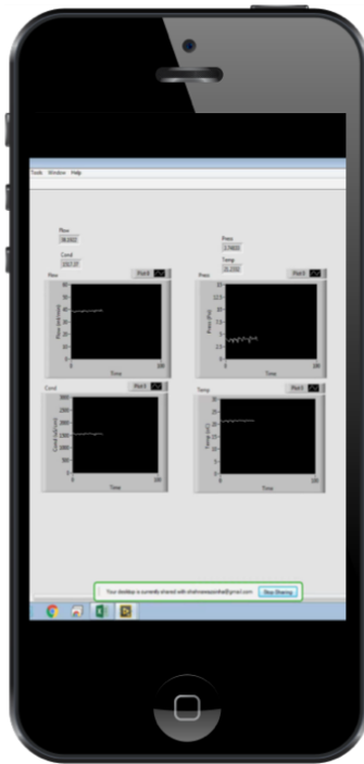
Figure 2.10: LabVIEW Data Remotely Viewed Using Google Chrome Remote Desktop Application and a Smartphone
