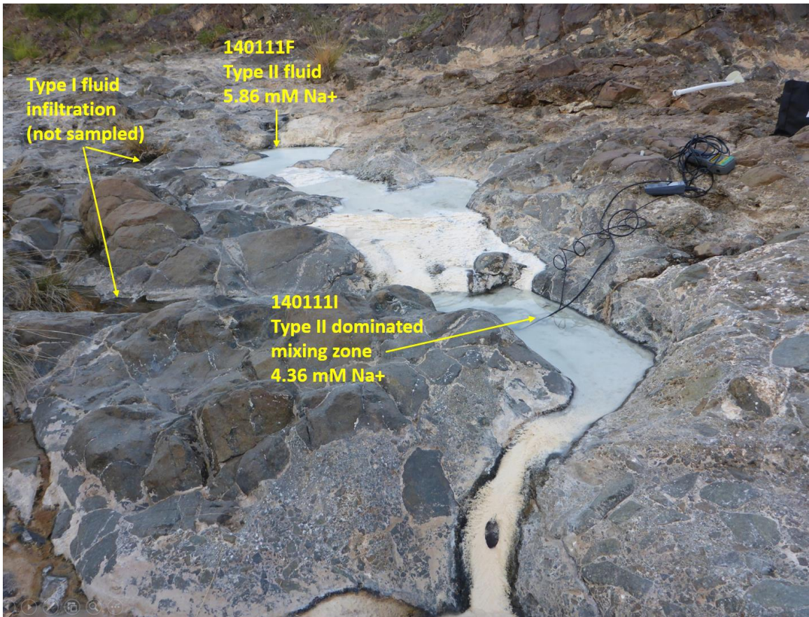
Fig. D2. Picture of Type II dominated fluid region of single mixing zone. Sample number and \text{Na}^+ concentrations are shown, which correspond to values in Table D3.
