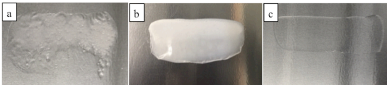
Figure 2-6. Addition cure PDMS film made with (a) 4,5-dichloroimidazole (dcIm) and (b) zinc acetate dihydrate and (c) pure PDMS. Note the white spots in (a) which are dcIm and note that a membrane film was not formed in (a), only a gel that could not be picked up in a single piece from the casting plate.
