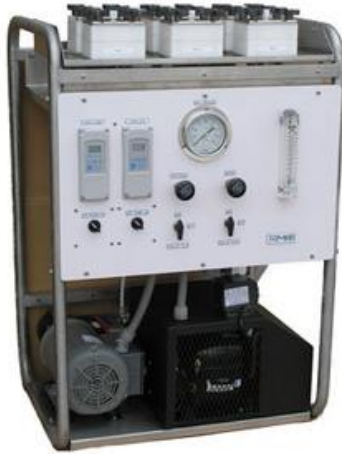
Figure 2.3 Cross-flow Test System
