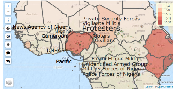
Figure 12. The comparison entity lens on the map shows the most frequently appearing actors from the ACLED dataset and the most frequently appearing named entities from the RSS news dataset. The area under the lens is used to filter the geocoordinates of all ACLED events and RSS news articles. After filtering the articles and extracting the relevant information from each dataset the RSS news' entities are shown on the left and ACLED events' actors are shown on the right.
