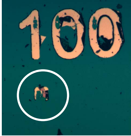
Fig. 4.36: MOS capacitors with 5 nm of chromium and 76 nm of gold gates were used for the gold wire bonding experiment. The metal gate film thickness was inadequate as the impact of pressure and ultrasonic energy during the thermosonic wedge bonding process caused the gate to peel off (marked within the white circle).
