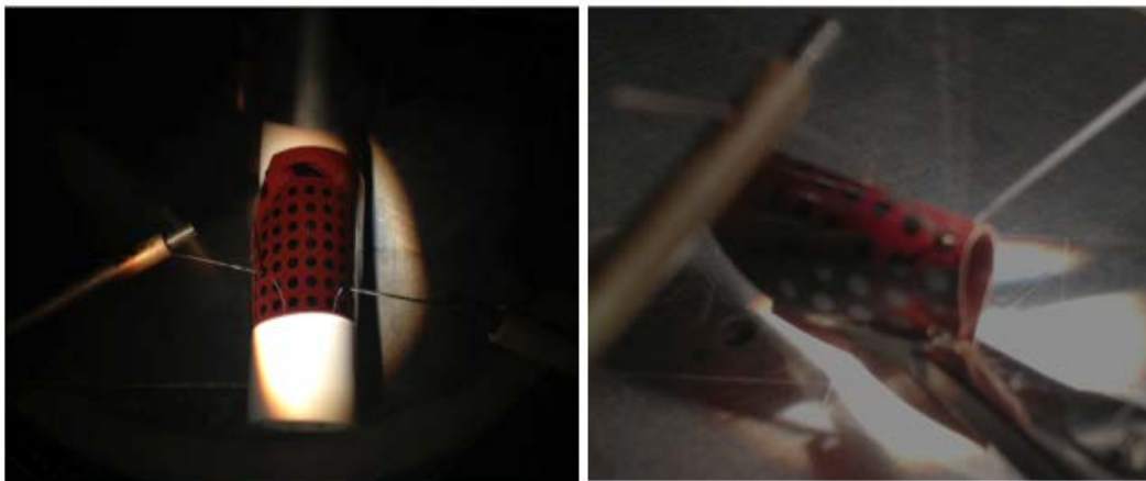
Fig. 3.13: Resistance measurement of Exp. A. sensor arrays while subjected to mechanical stress.
