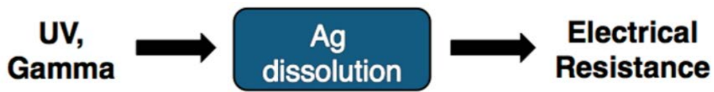
Fig. 3.1: ChG sensor overview: When the ChG sensors are exposed to ionizing radiation, the deposited energy causes Ag dissolution in ChG and the resulting resistivity change can be detected by the electrical resistance at the output.
