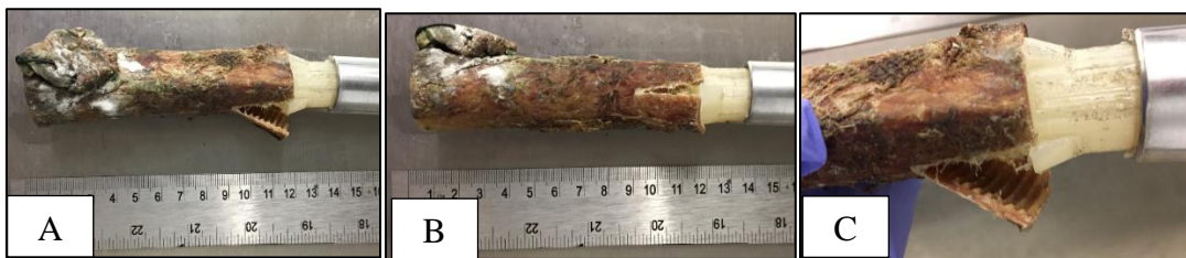
Figure 9. (TOP) Torque to failure and creep testing. Series 1 is the cadaver sample and series 2 is the simulated steel nut sample. (BOTTOM) Peak torque was observed when cadaver sample failed (A, B, C) not osseointegration screw.
