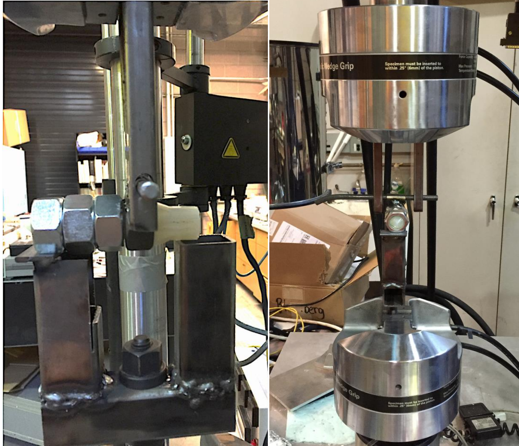
Figure 2. Three-point bending test fixture for FFF 3D printed osseointegrated screw.
